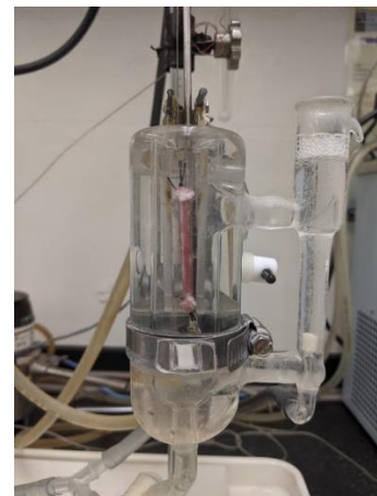
Figure 1. Isolated tissue bath containing a diaphragm muscle bundle attached to both force transducer and stationary hook and flanked by platinum stimulating electrodes.
