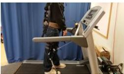
We have also developed a prototype of the automated gait training device using a servomotor and controller (left figure). The servomotor pulls and release the cable according to the angular movement profile of the
