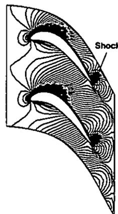
Fig. 9: Mach contour 8. blade row (midspan)
