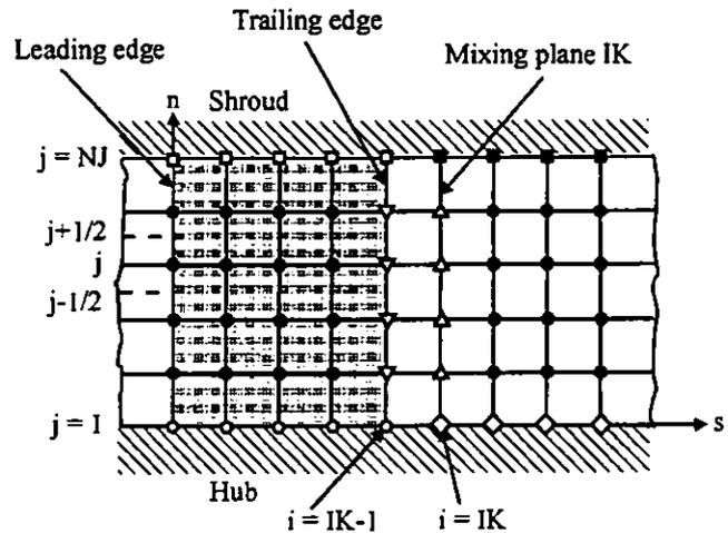
Fig. 4: Schematic section of the computational grid of the  $S_{2m}$ -stream surface
