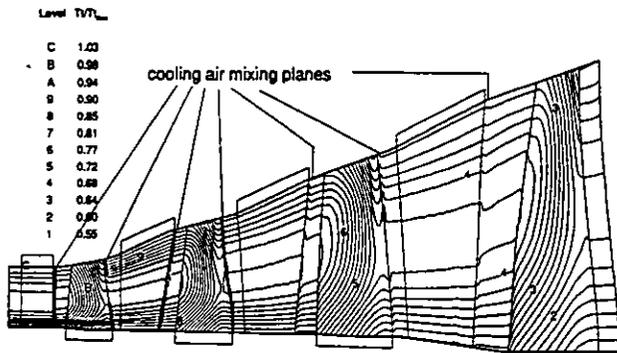
Fig. 11: Computed total temperature contour
