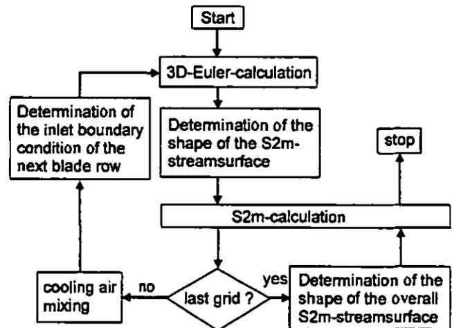
Fig. 3: Flowchart of the Q3DM-algorithm
