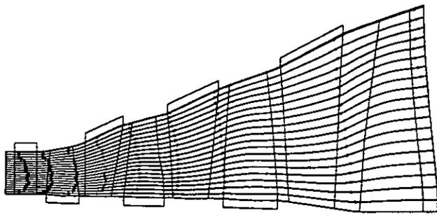
Fig. 10: Computed streamlines on  $S_{2m}$ -stream surface
