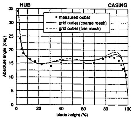
(a) Pitch angle  $\alpha$  at the cantilevered stator outlet.
