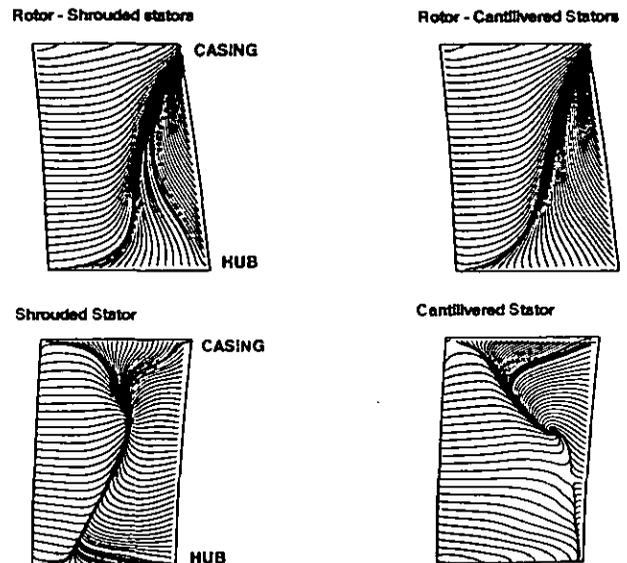
Figure 13: Flow visualizations on rotor and stator suction sides from isolated row calculations (near stall conditions).
