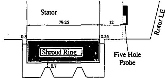
Figure 3: Build 1 shroud box, sealing and gap sizes (measures in mm).
