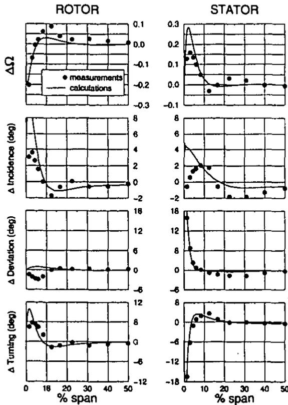
Figure 9: Computed and measured differences of losses, incidence, deviation and turning for the third stage rotors and stators between cantilevered and shrouded builds ( $\Delta = \text{cantilevered} - \text{shrouded}$  quantities).
