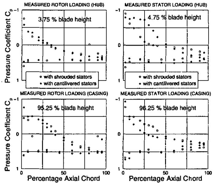
Figure 12: Measured static pressure coefficient  $C_p$  on rotor and stator blade near endwalls (near stall conditions).
