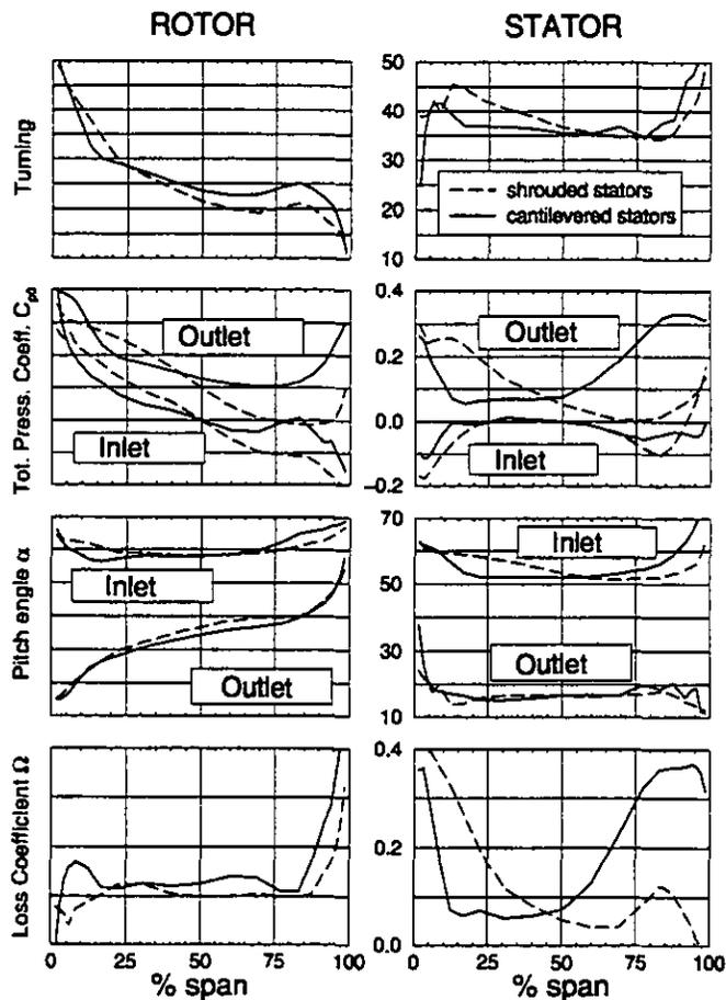
Figure 14: Measured turning, total pressure coefficient  $C_{p0}$ , pitch angles  $\alpha$  and losses  $\Omega$  in the third stage for both stator configurations.
