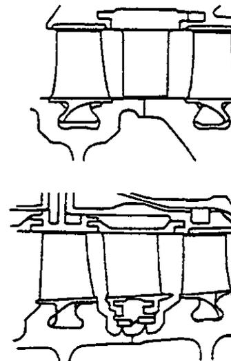
Figure 15: Schematic lateral view of cantilevered and shrouded stator hub of a real axial compressor.
