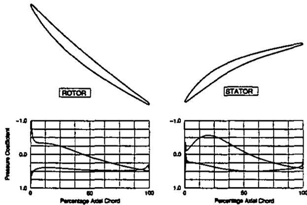
Figure 2: Rotor and stator profiles at midspan and their typical loading distributions at design operating conditions.
