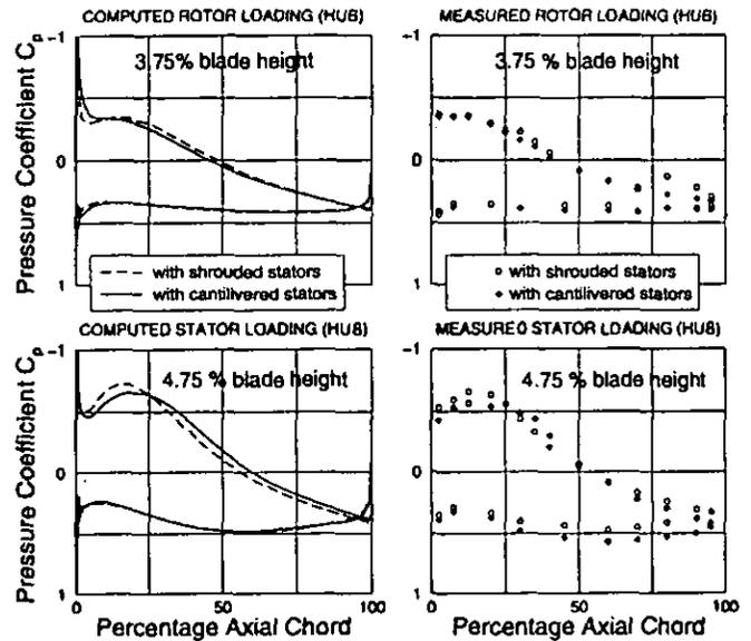
Figure 10: Computed (multistage) and measured static pressure coefficient  $C_p$  on rotor and stator blade near hub (design conditions).
