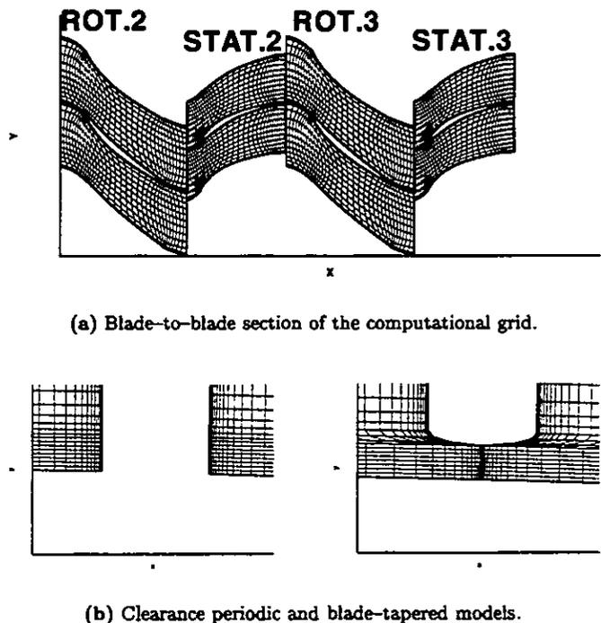
**Figure 4:** Details of the computational grid and clearance model.
