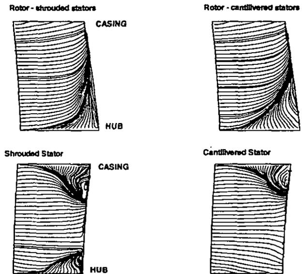
Figure 8: Flow visualizations on rotor and stator suction sides from isolated row calculations (design conditions) using measured data as inlet boundary conditions.
