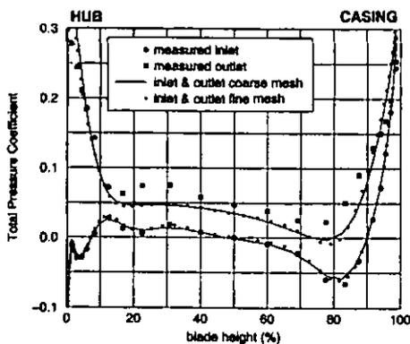
(b) Total Pressure Coefficient  $C_{p0}$  at the cantilevered stator inlet and outlet.
