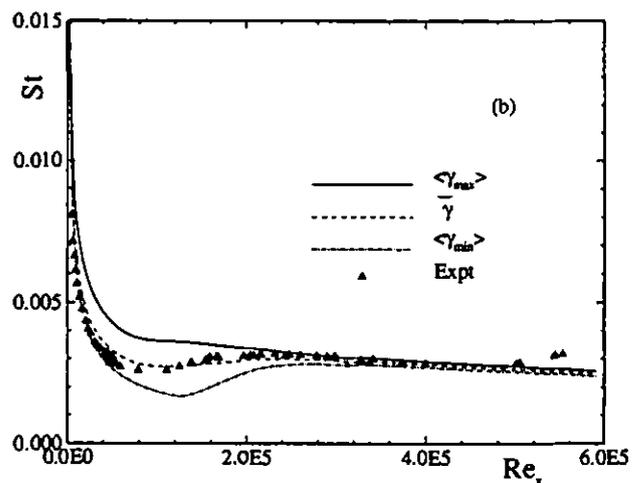
Figure 13(a and b). Heat transfer coefficients as a function of axial Reynolds number for (a)  $\Omega = 1.033$ (3-rods) and (b)  $\Omega = 5.166$ (15-rods).
