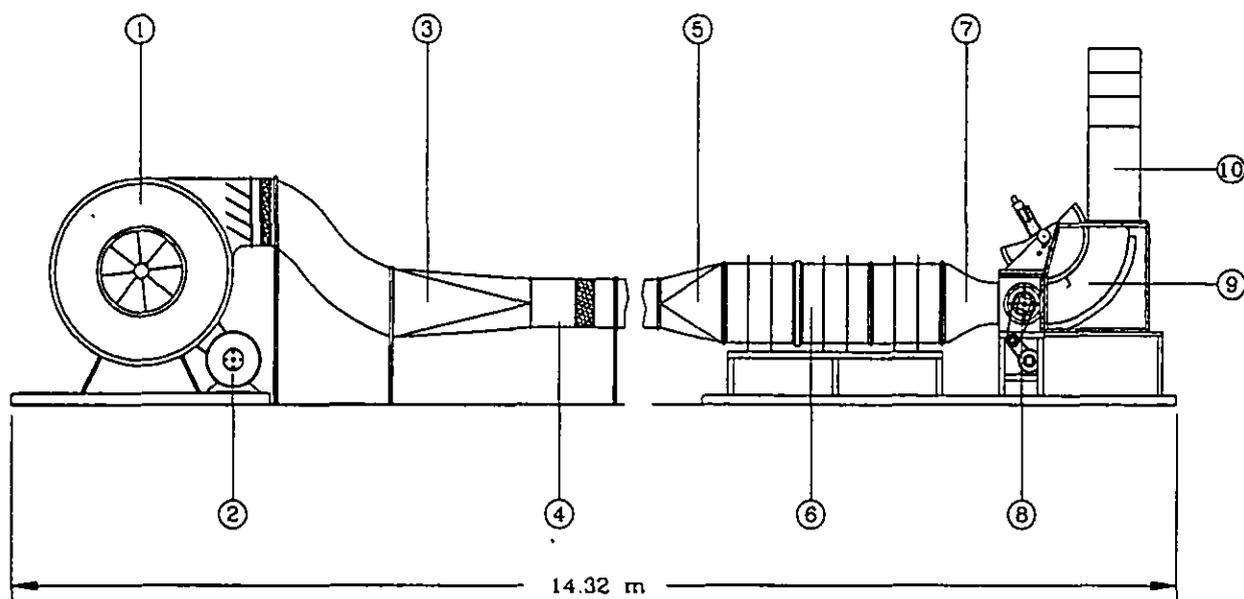
Figure 1. Overall layout of the test facility: 1. Fan, 2. Motor, 3. Transition duct, 4. Straight pipe, 5. Diffuser, 6. Settling Chamber, 7. Nozzle, 8. Wake generator, 9. Test section, 10. Exit duct.
