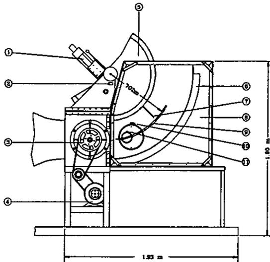
Figure 2. Test Section: 1. Traversing system, 2. Nozzle, 3. Wake generator, 4. Electric motor, 5. Convex wall, 6. Concave wall, 7. Hot-wire probe, 8. Plexiglass wall, 9. Curved plate, 10. Small vernier, 11. Large Vernier.
