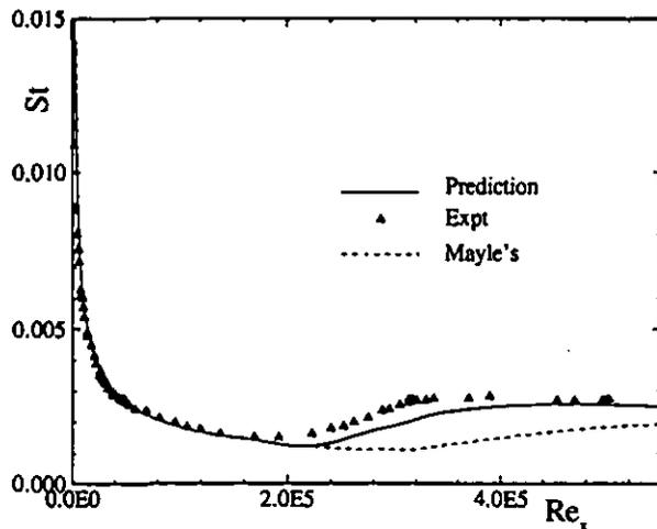
Figure 12. Heat transfer coefficients as a function of axial Reynolds number for no-rod or steady case.
