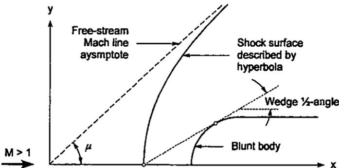
Figure 4. Detached shock waves approximated by Moeckel (1949) method
