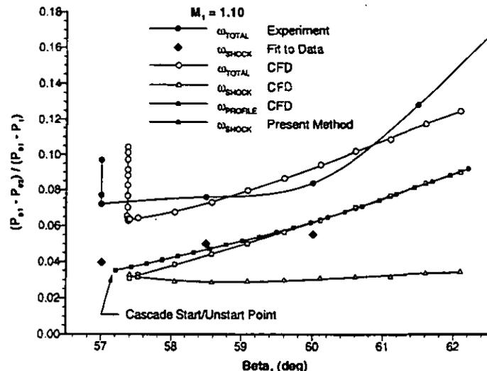
Figure 9. Loss coefficient comparison for unstarted operation of the L030-4 cascade with  $M_1 = 1.10$
