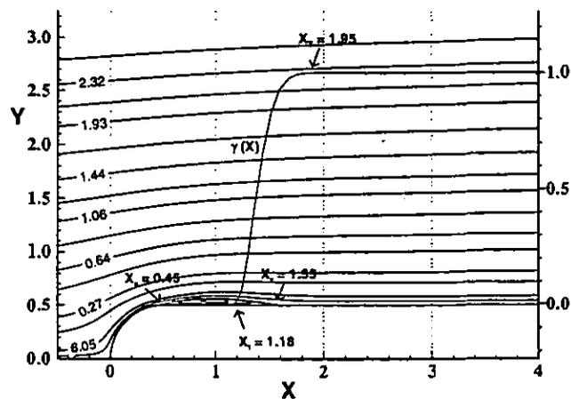
Fig. 8: Streamlines and intermittency distribution  $\gamma(X)$  for case 1f ( $U_i = 10 \text{ m/s}$ ,  $Tu_{\infty,s} = 2.5 \%$ .)
