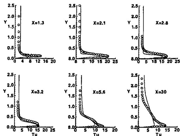
Fig. 7: Turbulence Intensity  $\sqrt{u'^2}/U_i$  profiles (%) for case 1c
