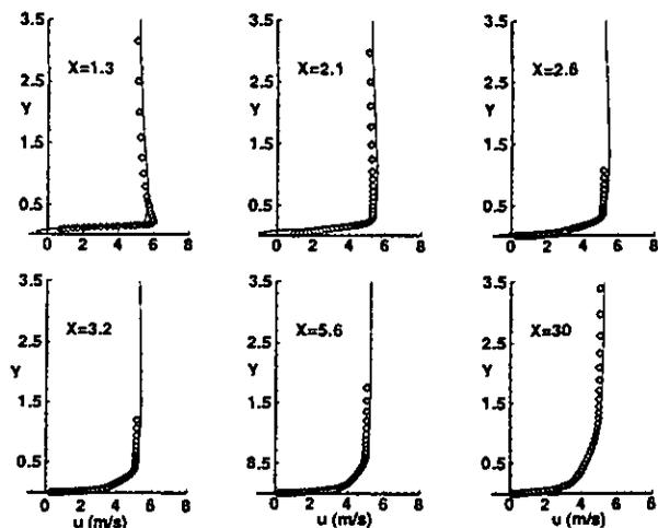
Fig. 6: Numerical (lines) vs. experimental (points) velocity profiles for case 1c.
