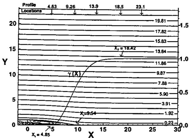
Fig. 13: Streamlines and intermittency distribution for testcase 2 ( $U_i = 11.38 \text{ m/s}$ ,  $Tu_\infty = 0.011 \%$ ).
