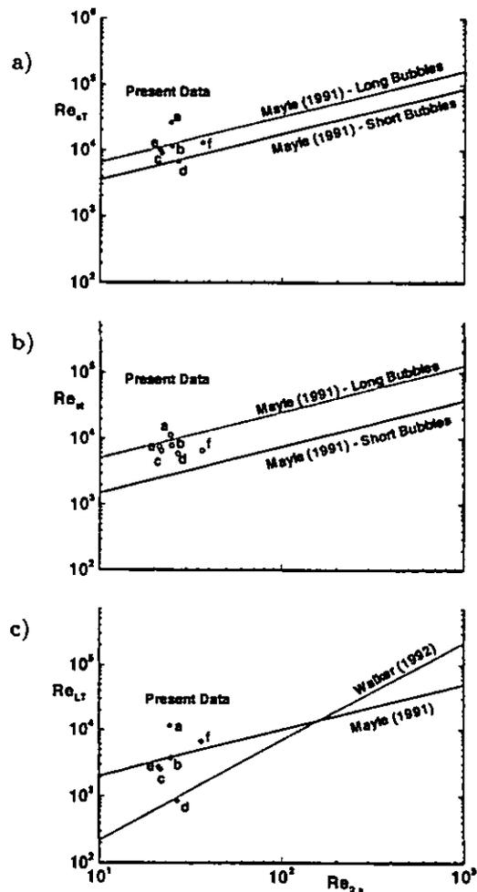
Fig. 12: Separation-bubble data for case 1 vs.  $Re_{2,s}$  and against available correlations. The ordinate  $Re$  is expressed in terms of : a) The length of the constant-pressure region ( $Re_{e,T}$ ), b) the distance between separation and transition points ( $Re_{e,t}$ ), c) the length of the transition region ( $Re_{e,L,T}$ ).
