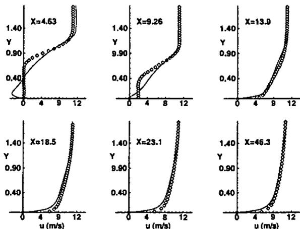
Fig. 16: Numerical (lines) vs. experimental (points) velocity profiles downstream of the step for testcase 2.
