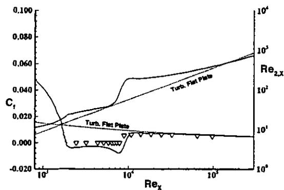
Fig. 5: Numerical (solid lines) vs. experimental results (points) and flat-plate correlations (dashed lines) for case 1c. Skin friction coefficient  $C_f$  and local  $Re_{2,x}$  are both plotted vs.  $Re_x$ .
