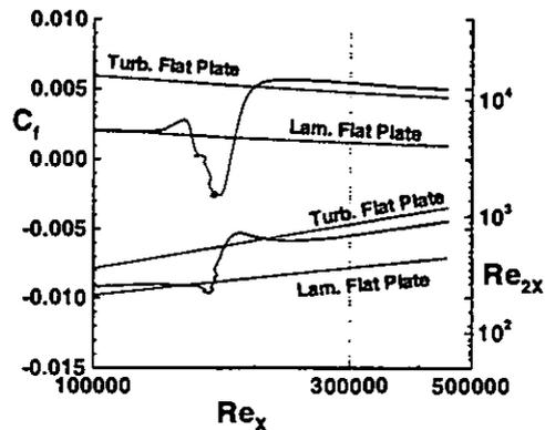
Fig. 15: Numerical results (solid lines) vs.  $Re_x$  and against flat-plate correlations (dashed lines) for testcase 2. Skin friction coefficient and momentum-thickness Reynolds number.
