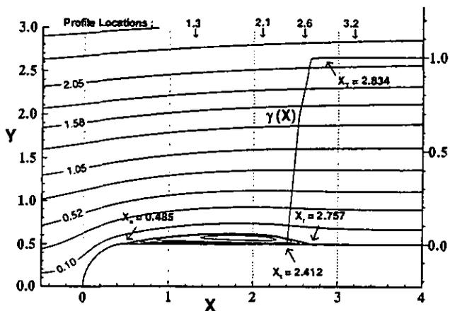
Fig. 3: Streamlines and intermittency distribution  $\gamma(X)$  for case 1c ( $U_i = 5 \text{ m/s}$ ,  $Tu_{\infty,s} = 2.31 \%$ .)
