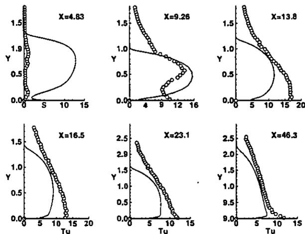
Fig. 17: Turbulence Intensity  $\sqrt{u'^2}/U_i$  profiles (%) downstream of the step for testcase 2.
