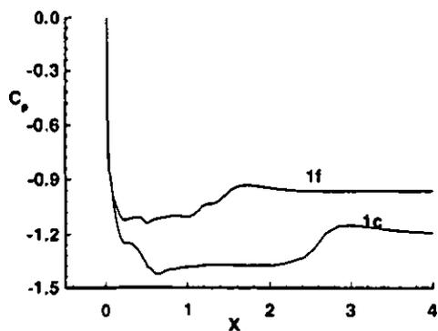
Fig. 11: Pressure Coefficient  $C_p$  vs.  $X$  for testcases 1c ( $X_t = 2.41$ ) and 1f ( $X_t = 1.18$ ).
