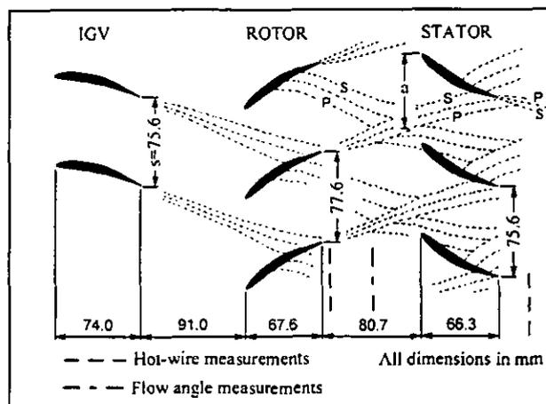
FIGURE 1: Cross-section of compressor blading at mid-passage, showing typical instantaneous wake dispersion. S = suction side; P = pressure side.
