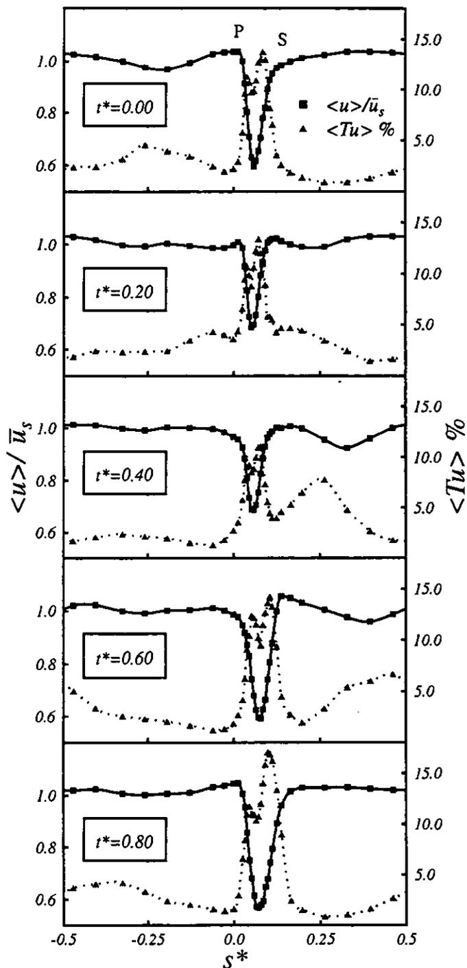
FIGURE 5: Typical variation in circumferential distributions of ensemble mean velocity and turbulence with phase of rotor wake passage. Hot-wire measurements 13.3% chord axially downstream of stator trailing edge at mid-passage.  $\phi = 0.675$ ,  $Re_{ref} = 120,000$ . S = suction side; P = pressure side.
