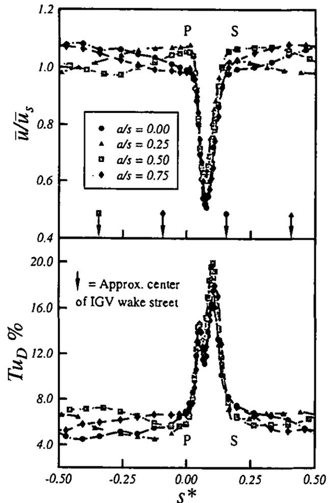
FIGURE 3: Influence of IGV clocking on circumferential variation of time mean velocity and total disturbance level. Hot-wire measurements 13.3% chord axially downstream of stator trailing edge at mid-passage.  $\phi = 0.600$ ,  $Re_{ref} = 120,000$ . S = suction side; P = pressure side.
