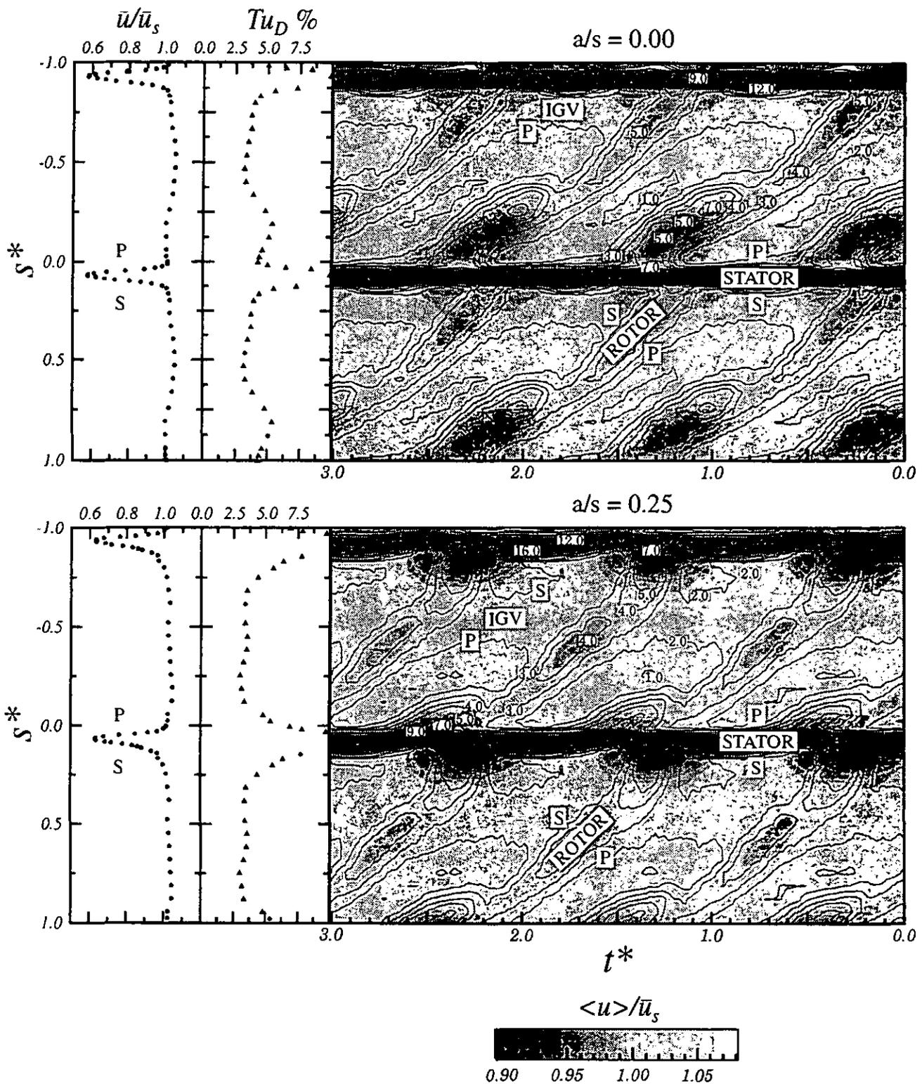
FIGURE 4: Influence of IGV locking on unsteady flow field downstream of stator. Hot-wire measurements 13.3% chord axially downstream of stator trailing edge at mid-passage.  $a/s$  indicates circumferential position of stator blades relative to center of IGV wake street. Line contours indicate ensemble average turbulence level,  $\langle Tu \rangle$  (%).  $\phi = 0.675$ ,  $Re_{ref} = 120,000$ . S = suction side; P = pressure side.
