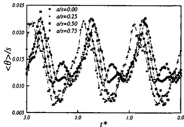
FIGURE 7: Influence of IGV clcking on temporal variation of ensemble average stator wake momentum thickness. Hot-wire measurements 13.3% chord axially downstream of stator trailing edge at mid-passage.  $\phi = 0.675$ ,  $Re_{ref} = 120,000$ .
