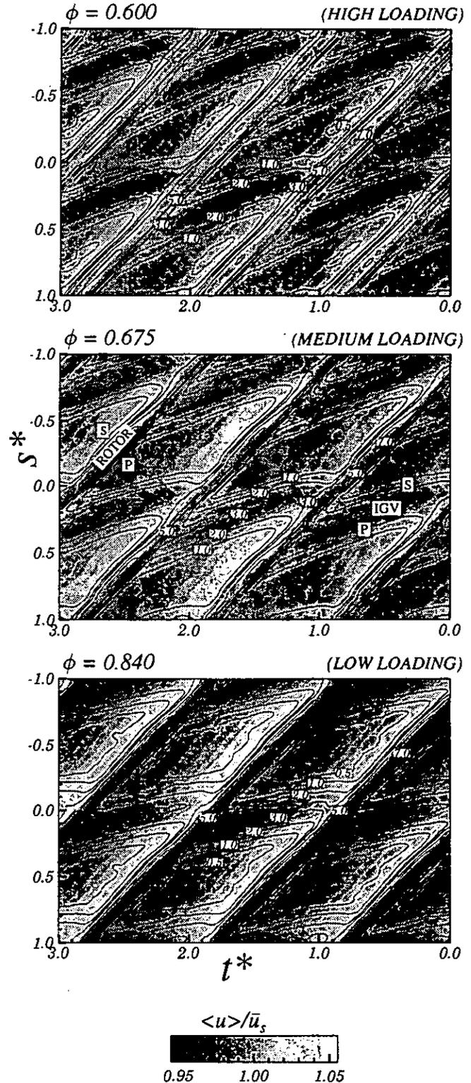
FIGURE 2: Variation of IGV wake dispersion with flow coefficient. Hot-wire measurements 5.5% chord axially downstream of rotor trailing edge at mid-passage. Line contours indicate ensemble average turbulence level,  $\langle Tu \rangle$  (%).  $Re_{ref} = 120,000$ . S = suction side; P = pressure side.
