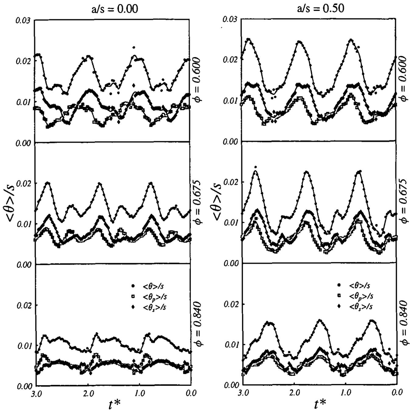
FIGURE 8: Temporal variation of stator wake momentum thickness 13.3% chord axially downstream of stator trailing edge at mid-passage, showing division into pressure and suction side components and influence of IGV clocking.  $Re_{ref} = 120,000$
