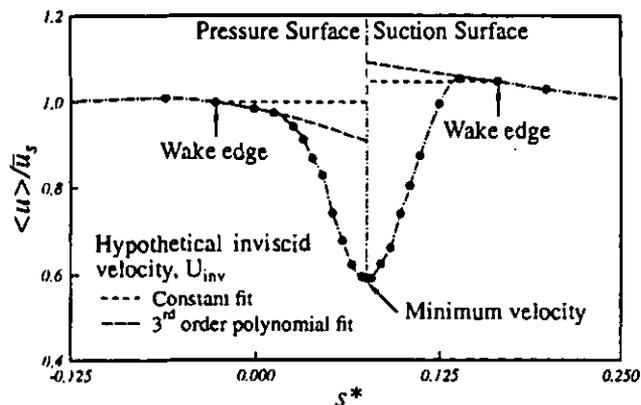
FIGURE 6: Alternative models for inviscid velocity distribution used for computing stator wake properties.
