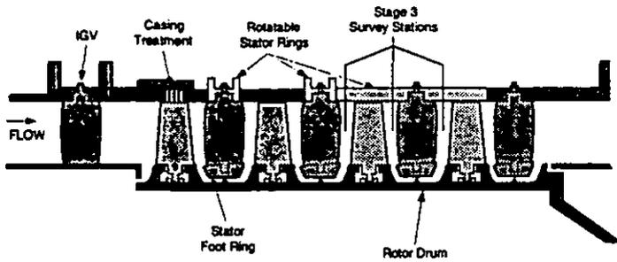
Figure 1 Schematic of NASA Low Speed Axial Compressor.
