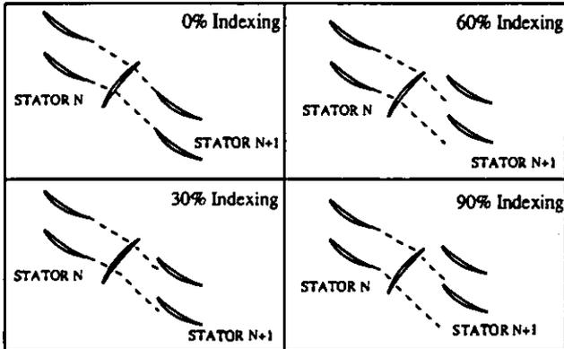
Figure 3 Stator Wake Indexing Alignment (Throughout Compressor).
