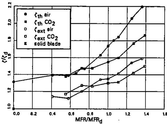
Figure 13: Global and external losses vs  $MFR$
