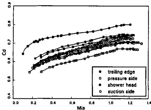
Figure 4: Discharge coefficients
