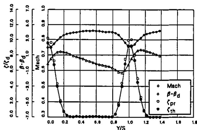
Figure 11: Downstream traverse- $MFR = 1.28MFR_d$
