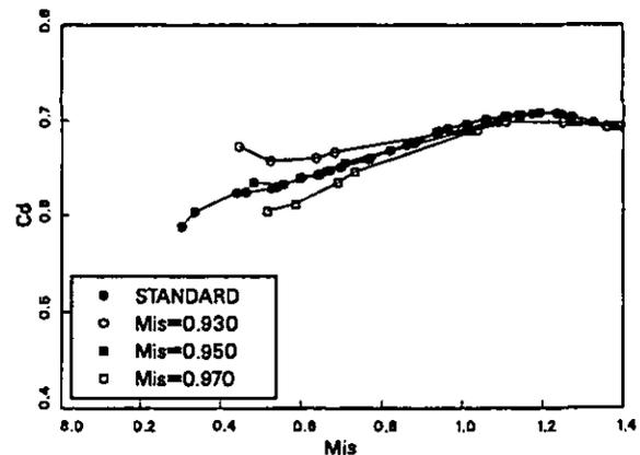
Figure 5: Discharge coefficient for hole n.12 for different assumed exit pressures
