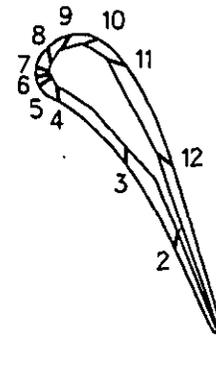
Figure 2: Film cooled nozzle guide vane
