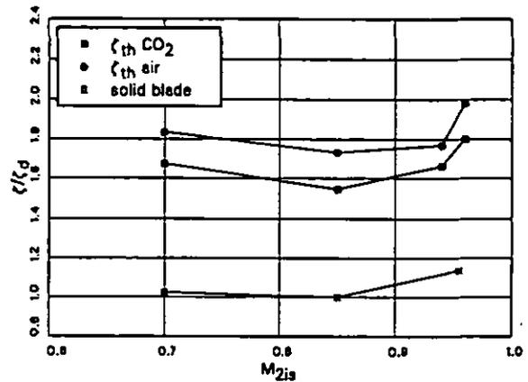
Figure 16: Losses vs.  $M_{2is}$  at  $MFR_d$
