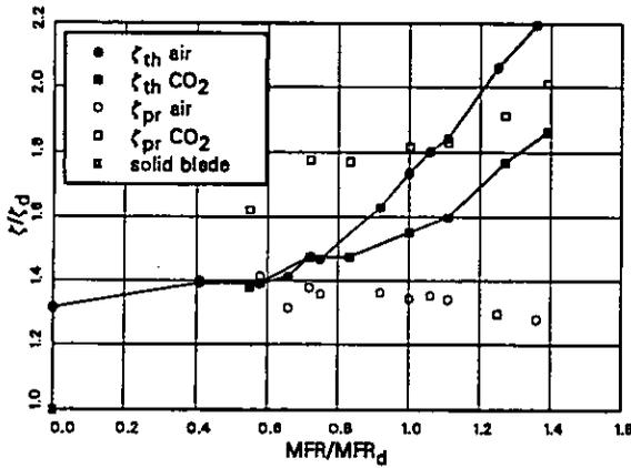
Figure 12: Losses vs. coolant mass flow rate
