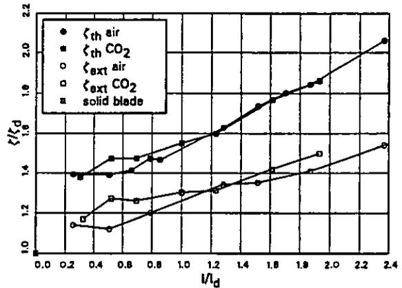
Figure 14: Losses vs. momentum flux
