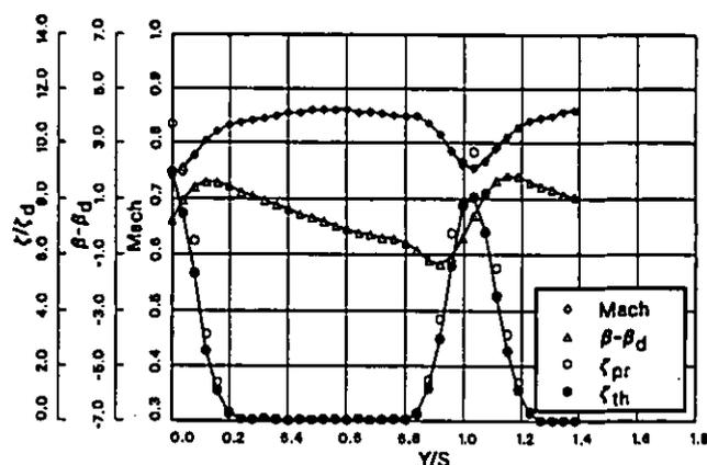
Figure 10: Downstream traverse-  $MFR = MFR_d$
