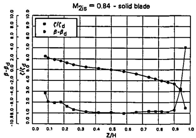
Figure 7: Spanwise loss and angle distributions
