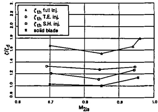
Figure 18: Losses vs  $M_{2is}$  at  $MFR_d$  for different injection modes
