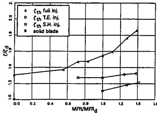
Figure 17: Losses vs.  $MFR_d$  for different injection modes
