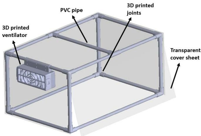
**FIGURE 1: THE STRUCTURE AND COMPONENTS OF VENTILATED PROTECTIVE TENT**
