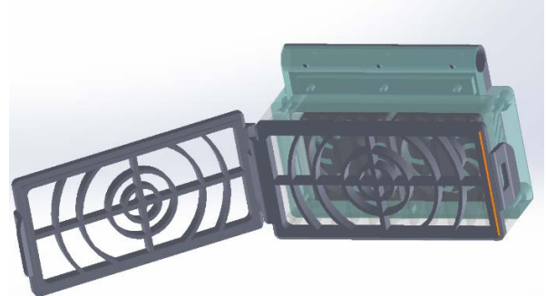
FIGURE 3: THE POSITIVE PRESSURE VENTILATOR SUPPLY CIRCULATED AIR TO THE TENT
