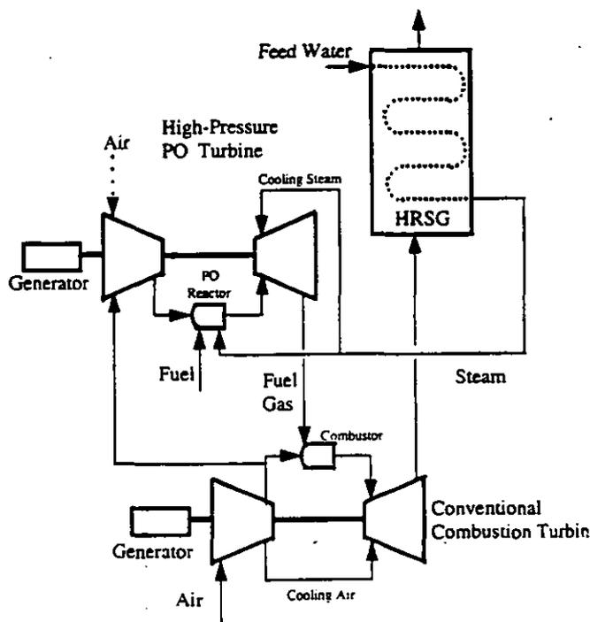
Figure 1 - Partial Oxidation Cycle Diagram
