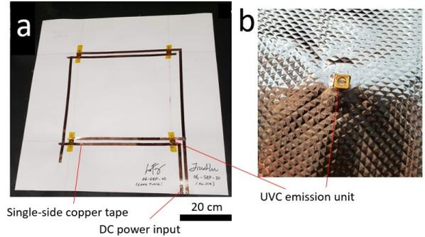
**FIGURE 2:** Test prototype: a) Image of non-reflective side of wrap featuring the diamond film sheet and copper tape wiring for 4 UVC emission units. b) Image of a UVC emission unit on the reflective side of the wrap.
