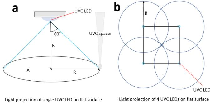
**FIGURE 4:** UVC LED Light Projection: **a)** UVC projection produced by a single UVC LED onto flat surface. **b)** UVC projected area by four UVC LEDs with a distance  $d = \sqrt{2}R = \sqrt{6}h$  between two adjacent LEDs.
