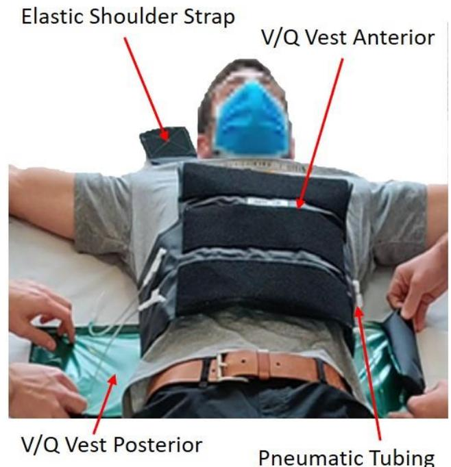
**FIGURE 1:** THE V/Q VEST APPLIED TO A RESEARCHER. THE VEST IS SPLIT INTO 3 PIECES TO SIMPLIFY APPLICATION TO A SEDATED PATIENT: THE ANTERIOR, LEFT POSTERIOR, AND RIGHT POSTERIOR. THERE ARE ELASTIC STRAPS AND VELCRO THAT SECURE THE VEST ONTO THE PATIENT AND RESTRICT THE VEST FROM EXPANDING AWAY FROM THE PATIENT.
