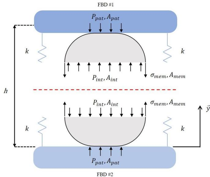
**FIGURE 4:** ILLUSTRATES THE EFFECT OF USING DIFFERENT STIFFNESSES OF ELASTIC USED TO RESTRICT THE EXPANSION OF THE BLADDERS AWAY FROM THE PATIENT. THE INTERNAL PRESSURE,  $P_{int}$ , REMAINS CONSTANT IN BOTH SCENARIOS AND  $k_2 > k_1$ . WITH HIGHER STIFFNESS ELASTIC, THE PRESSURE IMPARTED ON THE PATIENT IS INCREASED LIMITED TO THE INTERNAL PRESSURE OF THE BLADDER.
