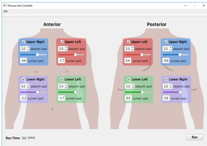
**FIGURE 6:** THE GUI DISPLAYED BY THE ELECTRO-PNEUMATIC CONTROLLER. A RASPBERRY PI 3 MODEL B IS USED FOR CONTROLLING AND DISPLAYING THE GUI.
