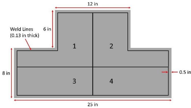
**FIGURE 3:** SHOWS THE WELD LINES CREATED BY THE IMPULSE SEALER. THE LEFT AND RIGHT SIDES OF BOTH THE ANTERIOR AND THE POSTERIOR OF THE VEST ARE CONNECTED WITH PNEUMATIC TUBING. THIS WAS DONE TO AVOID INTERIOR CORNERS THAT WEAKEN THE BLADDERS AND CAUSED THEM TO FAIL AT LOW PRESSURES.
