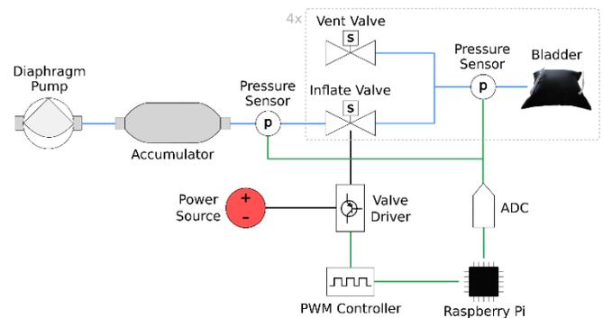
**FIGURE 5:** A CONTROL DIAGRAM FOR REGULATING THE INTERNAL PRESSURE OF THE INDEPENDENT BLADDERS THAT MAKE UP THE V/Q VEST.
