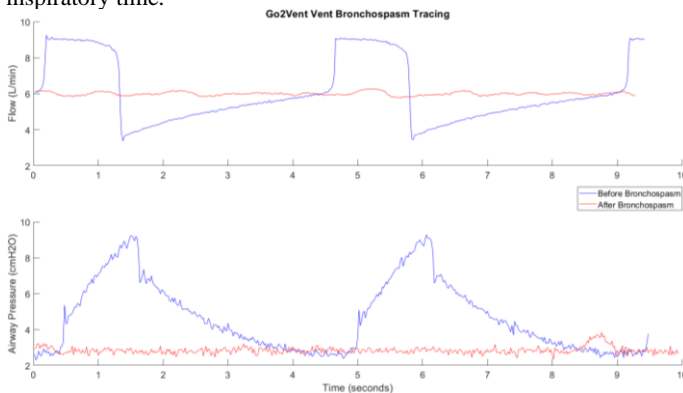
FIGURE 7: Go2Vent ventilator before and after Bronchospasm. Note that the ventilator is unable to produce adequate airway volumes after introduction of spasm without intervention.
