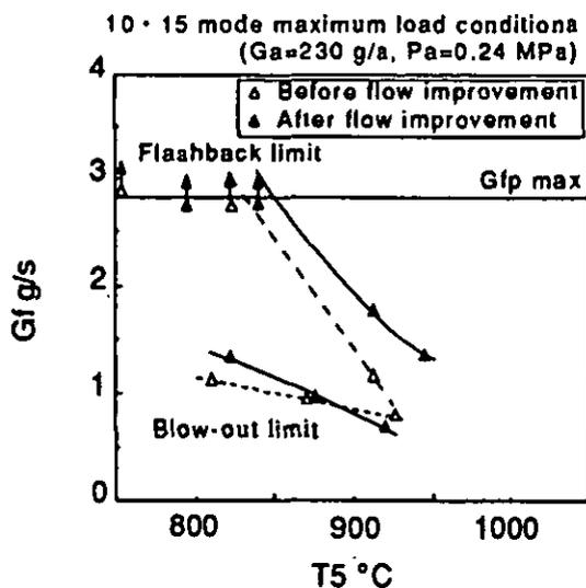
Figure 3 Combustor inlet temperature vs. stable combustion range
