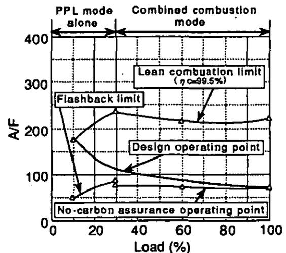
Fig. 8 Stable combustion range of the improved PPL-2 combustor
