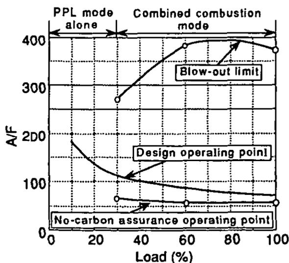
Figure 10 Stable combustion range of the A/F=60 type PPL-2 combustor
