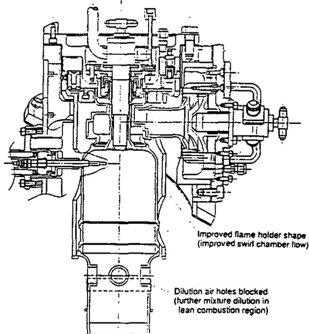
Figure 9 Construction of the A/F=60 type PPL-2 combustor
