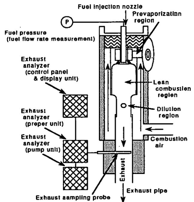
Figure 5 Schematic of transient emission test apparatus
