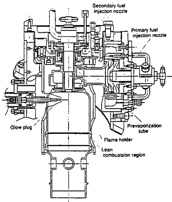
Figure 2 Construction of the PPL combustor
