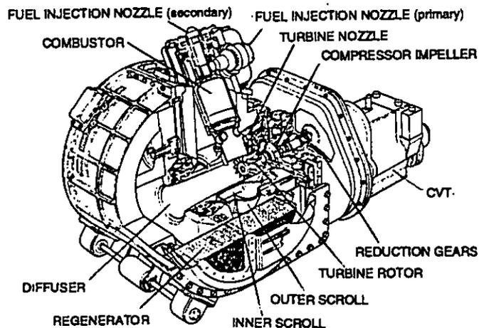
Figure 1 Construction of the 100-kW CGT engine
