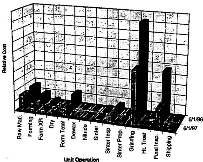
Fig. 9. KICC Cost Model For Ceramic Turbine Nozzles.
