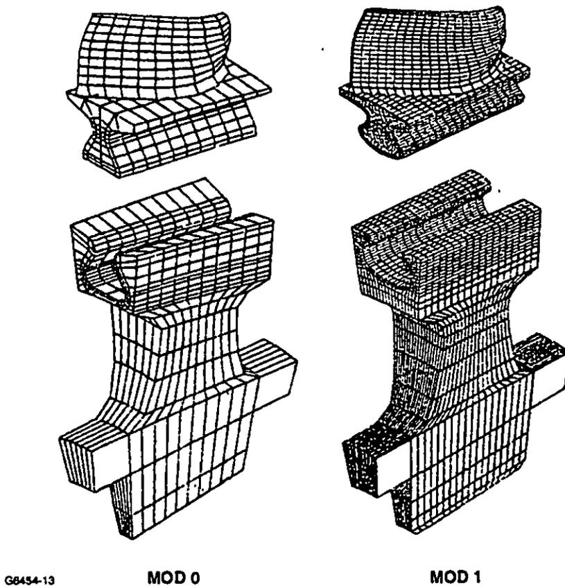
**Fig. 13. Finite Element Models Used For Ceramic Blade Attachment Frictional Analyses.**
