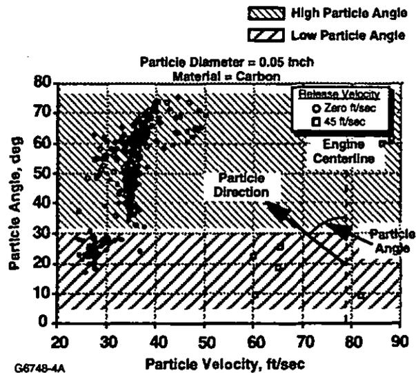
Fig. 4. CFD Analysis Indicates Particles Follow Two Distinct Paths Exiting The Turbine Stators.
