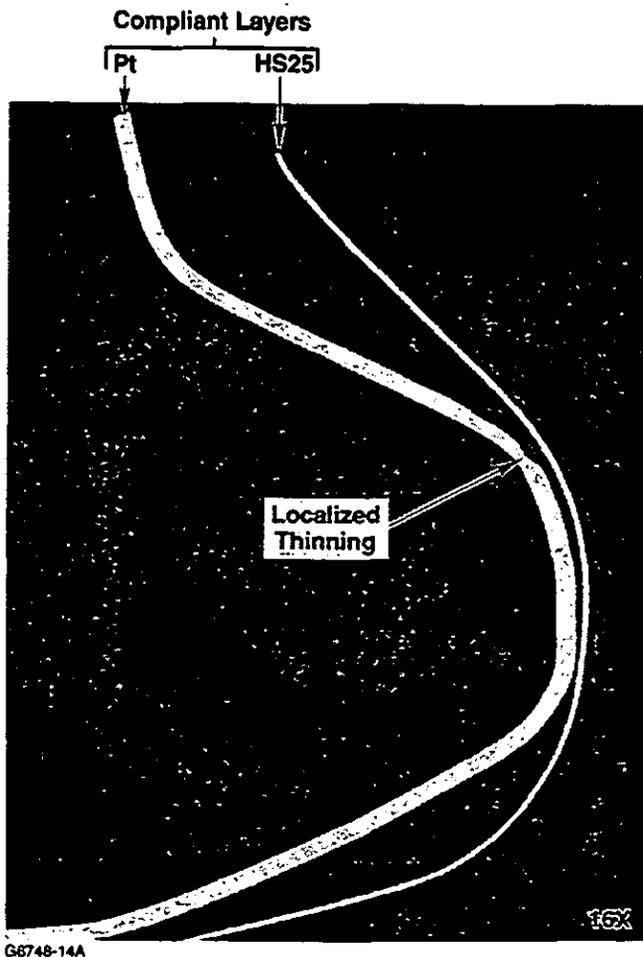
Fig. 12. Cross-Section Through Compliant Layers Following 125 Hours Of Operational Testing.
