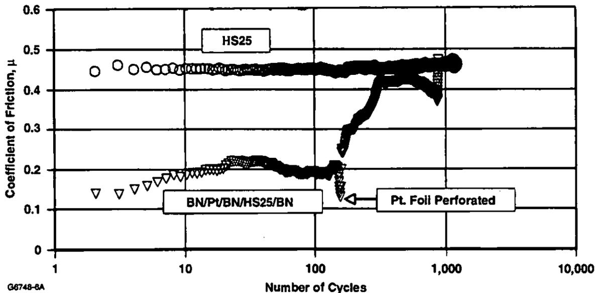
Fig. 6. High Temperature (1200F/649C) Screening Test Results Confirm Lubricated Dual Compliant Layer System Is Effective For Initial Ceramic Blade Engine Testing.
