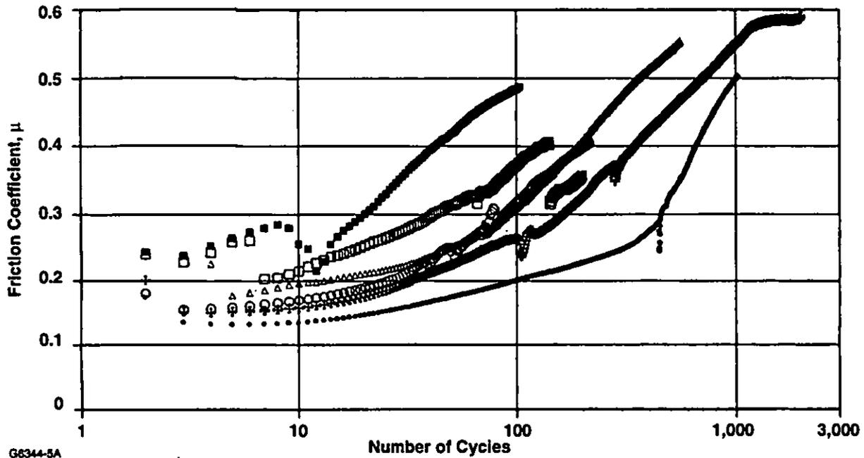
Fig. 5. Room Temperature Screening Test Results Show HS25 Compliant Layer Has Low Short-Term Coefficient Of Friction.
