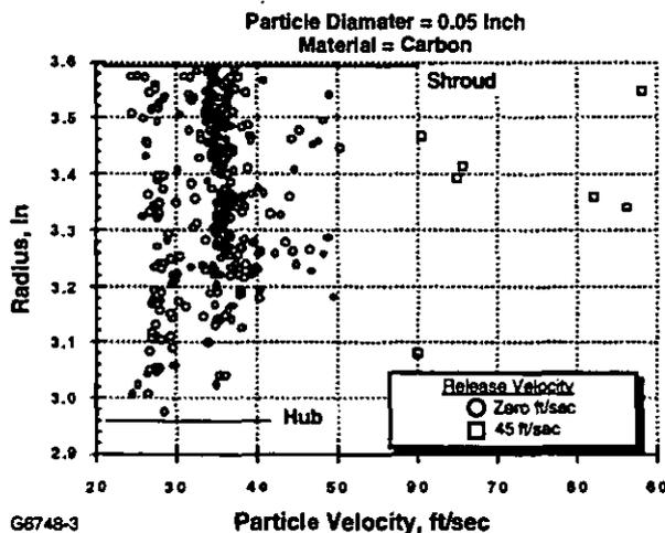
Fig. 3. Computed Particle Velocities Versus Turbine Flowpath Radius.
