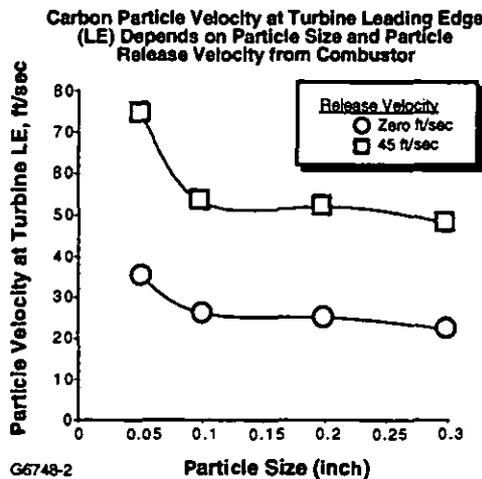
Fig. 2. Computed Particle Velocities At Turbine Blade Leading Edge Versus Particle Sizes.
