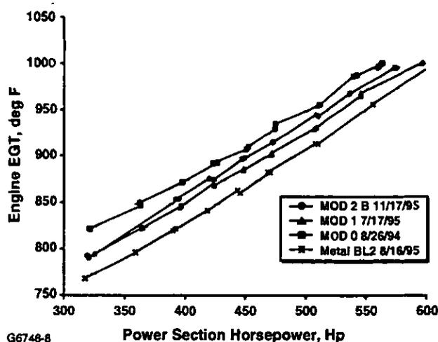
Fig. 10. 331-200[CT] Ceramic Nozzle Engine Performance Test Results.
