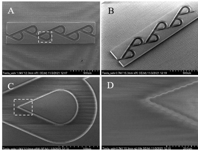
**FIGURE 2:** Scanning electron micrographs of 2D Tesla valve shown in (A) top view and (B) isometric view. Higher magnifications of the framed regions are shown in C and D.
