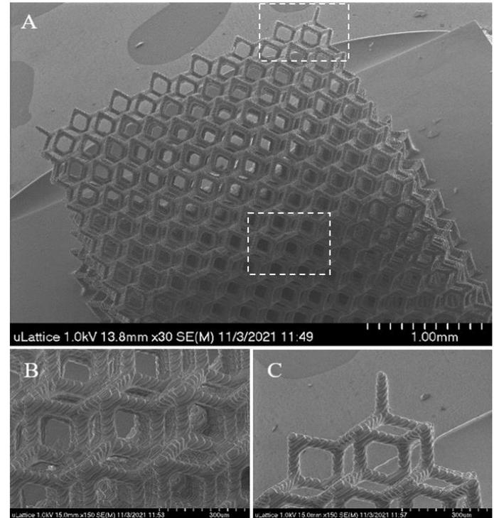
**FIGURE 5:** A: Scanning electron micrograph of the cubic fluorite microlattice; each individual unit cell with struts and perforations can be clearly identified. Close-up on the center (B) and corner (C) of the microlattice.
