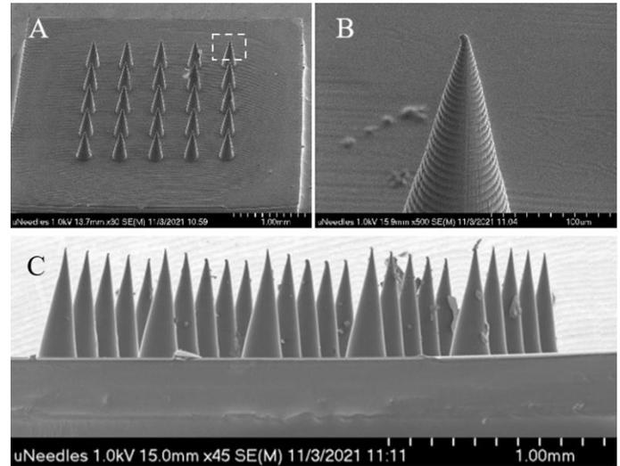
**FIGURE 4:** A: Scanning electron micrograph of the microneedle array. B: Scanning electron micrograph close-up on the tip of the microneedle framed in A; each indicial circular slice can be identified. C: Side view of the microneedle array. There are some impurities on the needles that probably occurred after the printing process.
