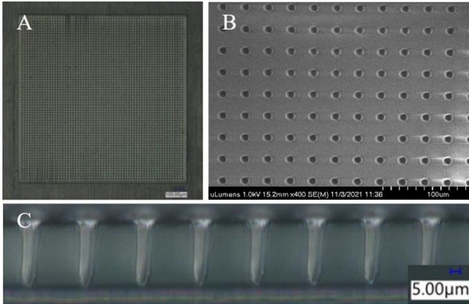
**FIGURE 3:** A: Digital light micrograph of the microlumen array at 40X magnification. B: Scanning electron micrograph of a section of the array at 400X magnification. C: Digital light micrograph showing the side views of the lumens that are penetrating down. As can be seen, the lumens are flat for the most part but taper down towards the bottom.
