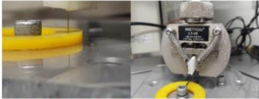
FIGURE 2: THE MICRONEEDLE IS CLAMPED AND SECURED TO THE INSTRON AND THE NEEDLE TIP IS IN CONTACT WITH THE DUROMETER
