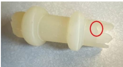
FIGURE 5: CRACKS OBSERVED IN ARD V1.
