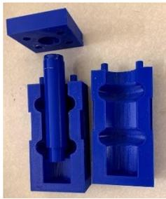
**FIGURE 1: THE MOLD USED FOR INJECTION MOLDING.**
