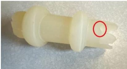
**FIGURE 5:** CRACKS OBSERVED IN ARD V1.
