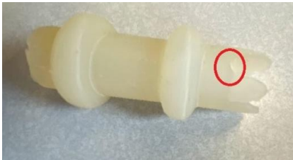
FIGURE 5: CRACKS OBSERVED IN ARD V1.
