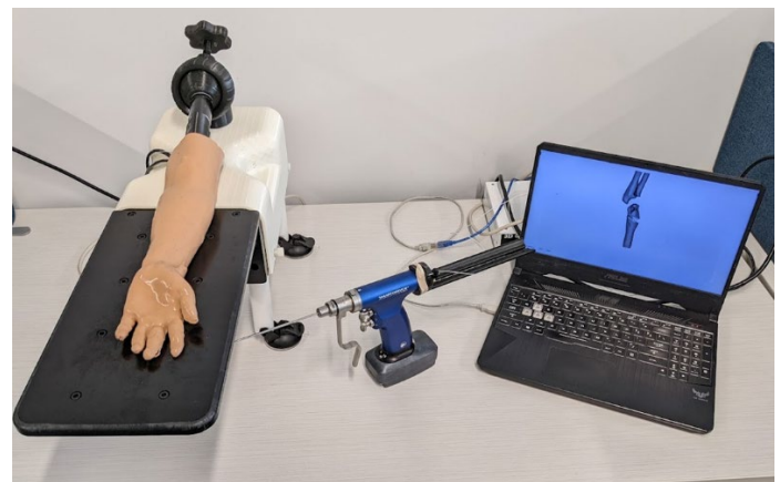
Figure 1: Simulator package including surgical model, surgical drill, and associated laptop.
