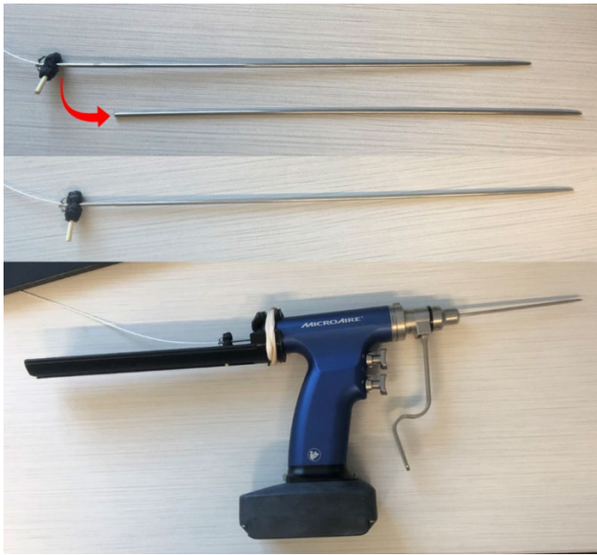
Figure 4: Surgical drill tracking. Stationary wire (top) inserts into the hollow wire that can freely rotate when inserted into the surgical drill (bottom).
