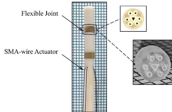
**FIGURE 1:** SMA-ACTIVATED MULTI-JOINT FLEXIBLE ACTIVE NEEDLE (LEFT), FLEXIBLE JOINTS; 3D PRINTED DIGITAL PHOTOPOLYMER, ©Proto Labs, INC. (RIGHT).
