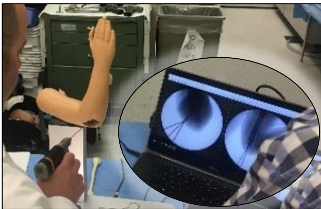
Figure 2: The prototype simulator in use. On the screen of the laptop are the generated corresponding synthetic fluoroscopic images (zoomed in inset image for sake of visualization).
