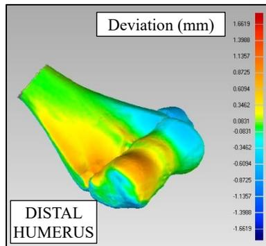
A large change in the mean deviation but small change in SD would suggest that placement of the bone into its holder is not repeatable. A large change in the mean deviation, but small
