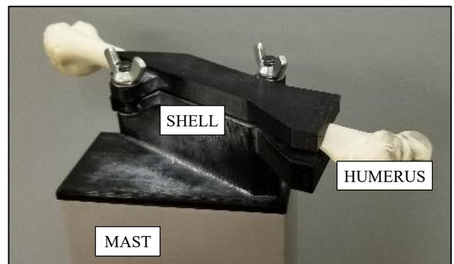
**Figure 3:** The prototype fixation method.
