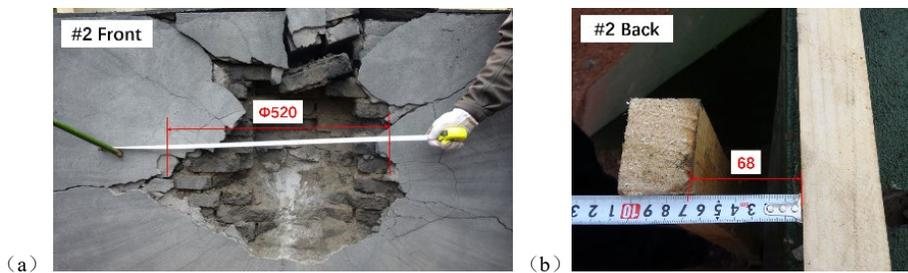
Fig 6. Impact fracture of back surface sprayed polyurea masonry walls (a) Front surface ; (b) Back surface
