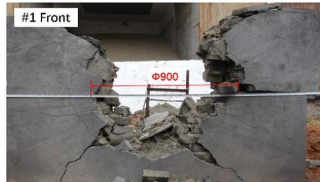
Fig 5. Impact fracture of non-sprayed masonry walls on the front surface
