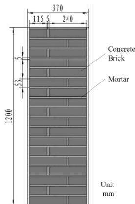
Fig 2. Structural dimensions of standard masonry walls
