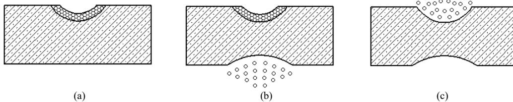
Fig.1. Impact process of a blast wave on the non-sprayed wall (a) Front surface of the wall is crushed after the compressional wave. (b) Back surface of the wall generates spallation after the expansion wave. (c) The crushed wall is thrown outward after the reflected wave.
