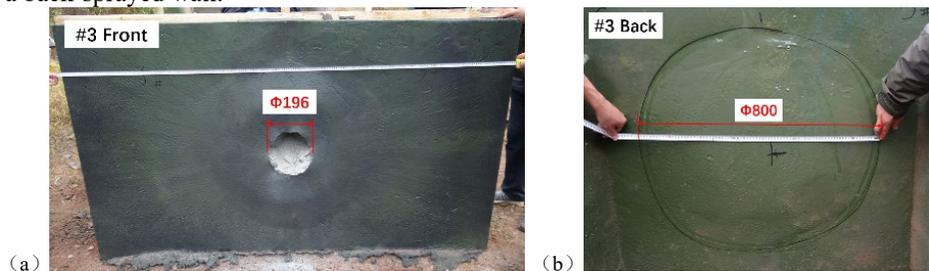
Fig 7. Impact fracture of double-sided polyurea sprayed masonry wall (a) Front surface ; (b) Back surface
