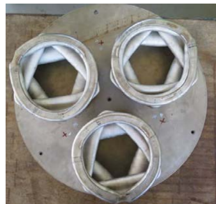
Figure 7: Deformed Shapes of Impact Limiter Tubes
