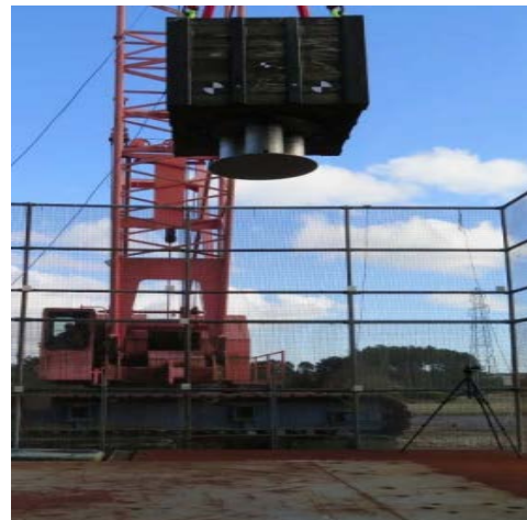
Figure 4: Assembled ILA Prototype/Drop Weight Pick Up by a Crawler Crane Before the Drop Test
