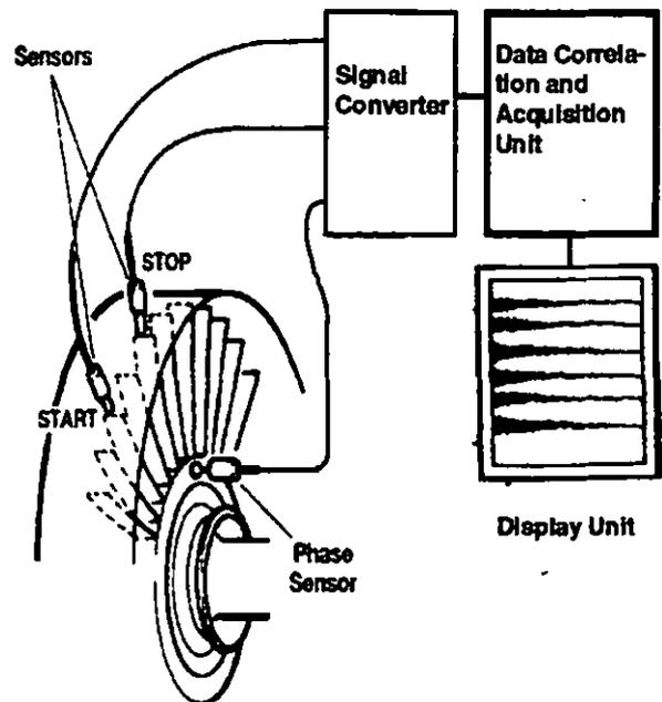
Figure 8: Schematic of the non-contact blade vibration measurement system
