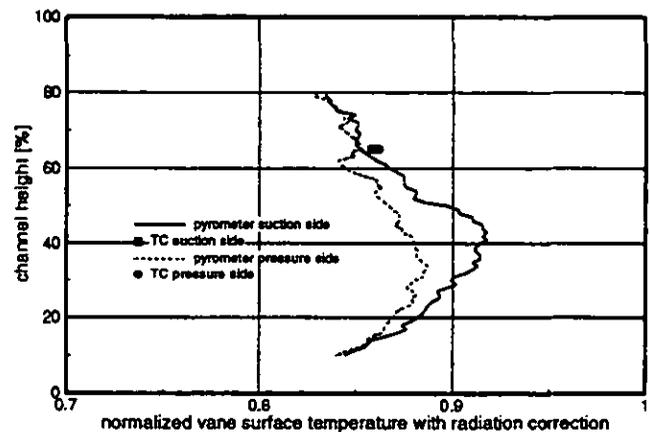
Figure 11: Typical vane temperature-profile of the second stage for two viewing angles
