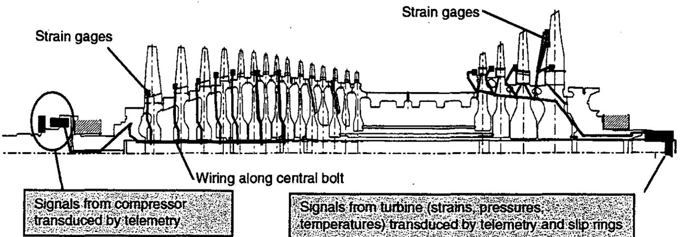
Figure 5: Schematic of the signal path in the rotor
