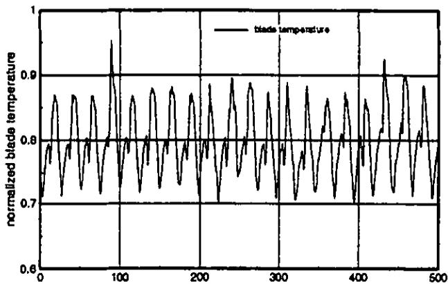
Figure 10: Typical blade temperature distribution for 20 first-stage blades
