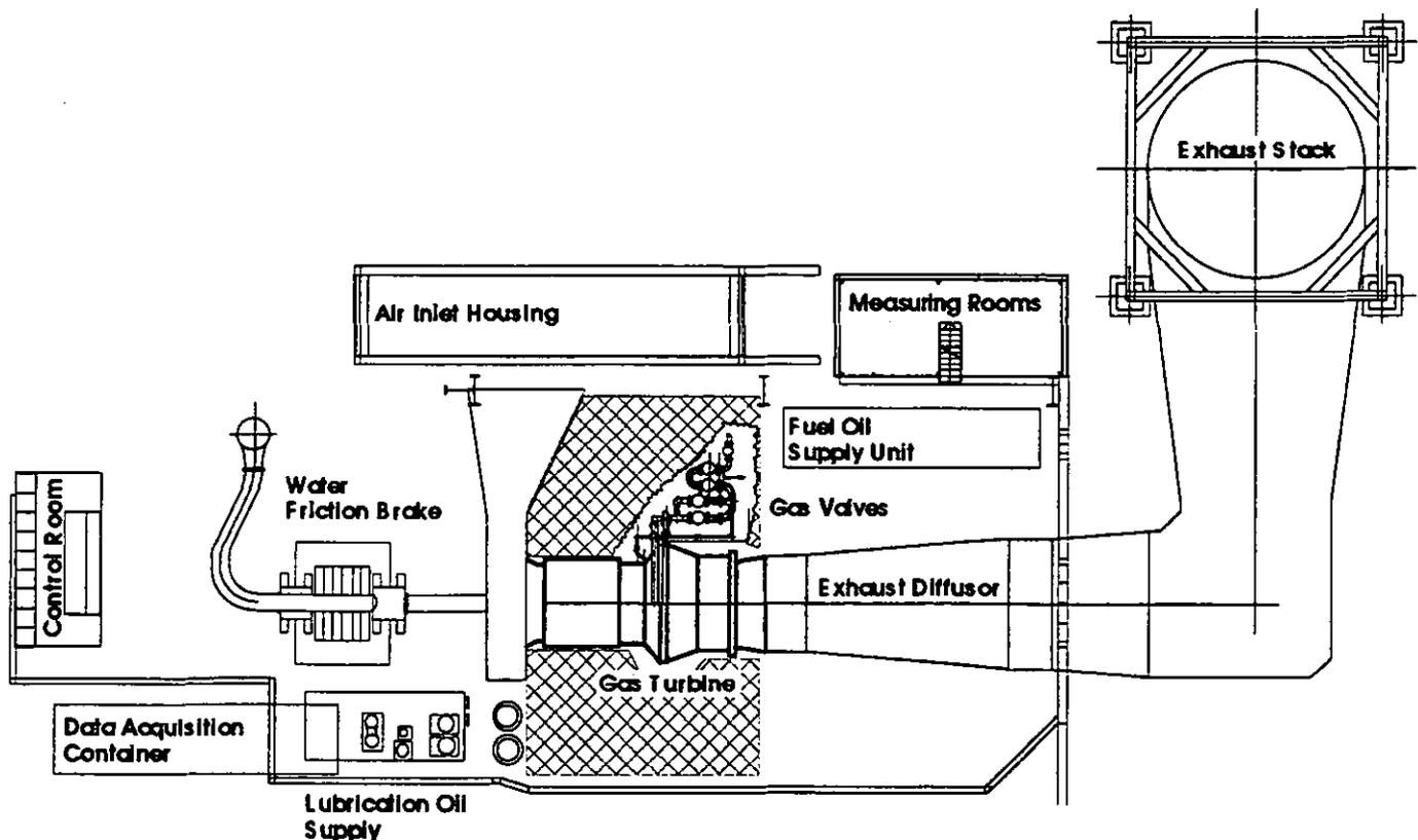
Figure 1: Layout of the test facility
