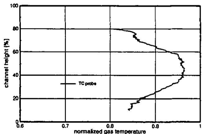
Figure 12: Radial temperature profile up-stream of the second stage
