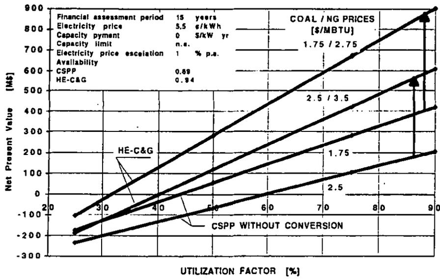
Fig. 14 - The Net Present Value (NPV) vs. utilization factor with and without conversion into HE-C&G with 1xGT26 of a 500 MW coal-fired CSPP.
