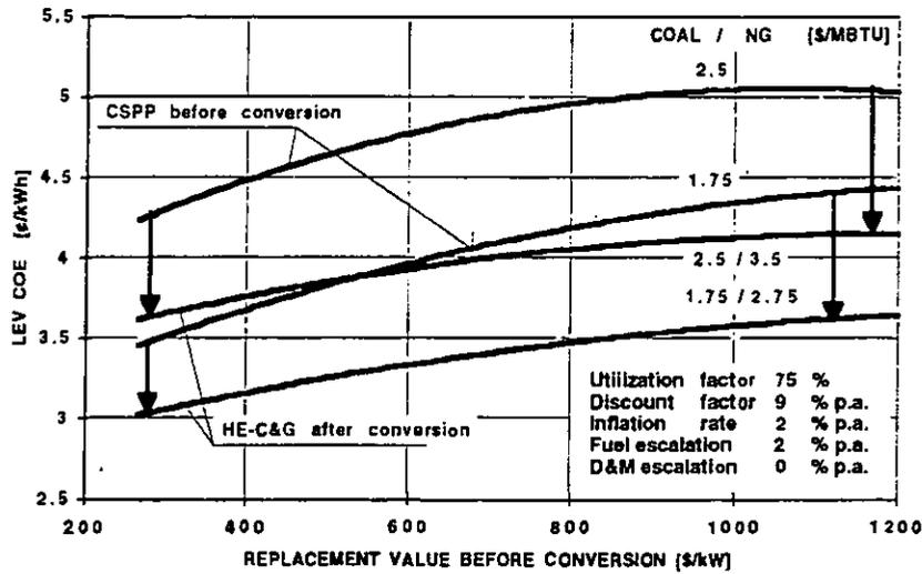
Fig. 10 - Comparison of LEV COE before and after conversion into HE-C&G vs. initial CSPP Replacement value .
