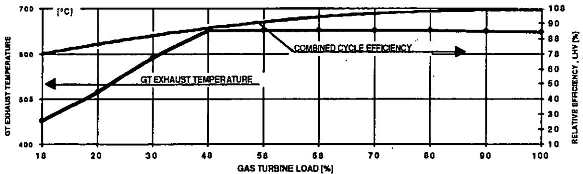
Fig. 2 - GT24/GT26 exhaust gas temperature and combined cycle part load efficiency versus gas turbine load characteristic .
