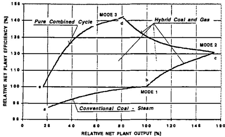
Fig. 4 - Efficiency versus load characteristic of a 500 MW CSPP converted into HE-C&G with 1xGT26. The *Operating Domain* is defined inside the surface limited by the curves ab-bc-cd-de with ab - conventional mode ; bc , cd and the surface inside the operating domain - hybrid , coal and gas and de - pure combined cycle mode
