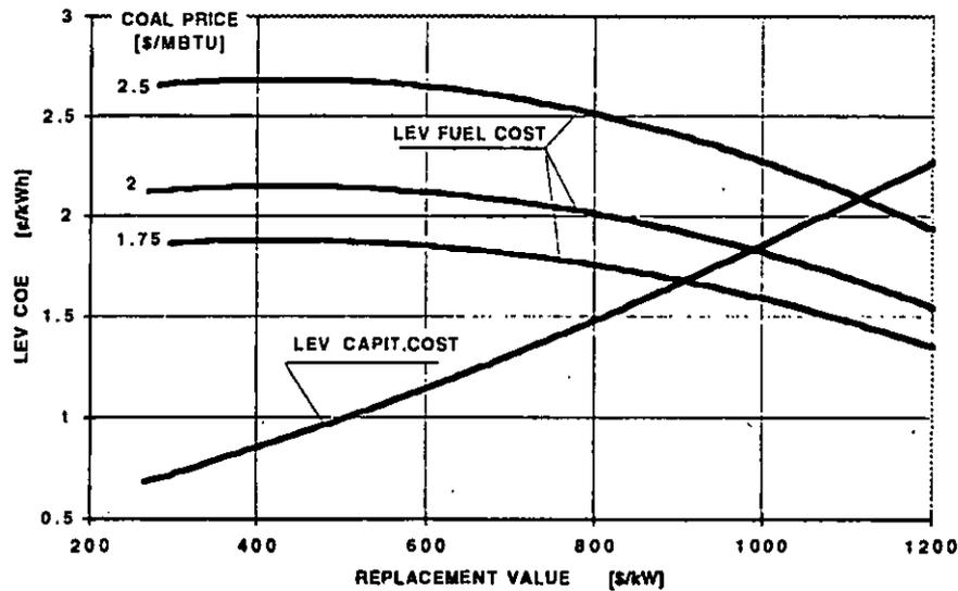
Fig. 8 - The levelized generating cost breakdown : fuel and capital costs of Steam Power Plants with different Replacement values before conversion into HE-C&G .
