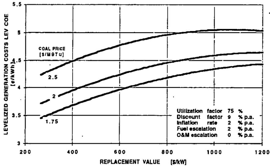
Fig. 7 - Levelized electricity generating costs (LEV COE) of Steam Power Plants with different Replacement values before conversion into HE-C&G .
