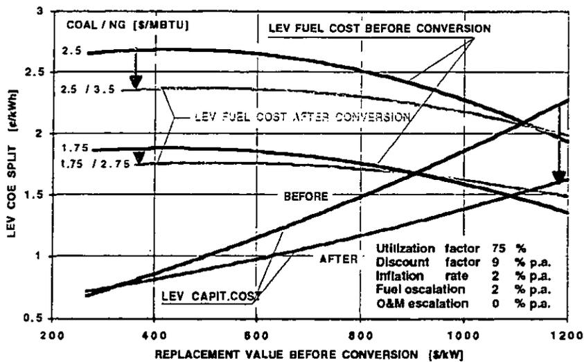
Fig. 11 - Comparison of levelized fuel and capital cost before and after conversion into HE-C&G with 1xGT26 vs. initial Replacement value .
