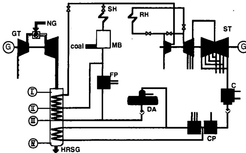
Fig. 3 - Principle of the High Efficiency Coal and Gas (HE-C&G) : integration of a Sequential Combustion gas turbine GT24/GT26 and HRSG with a Conventional Steam Power Plant (CSPP) : MB - Main Boiler; SH - Superheater ; RH - Reheater ; ST - Steam Turbine; C - Steam Condenser ; CP - Condensate Preheaters; DA - Deaerator ; FP - Feedwater Preheaters; HRSG - Heat Recovery Steam Generator ; GT - Gas Turbine; NG - Natural Gas .
