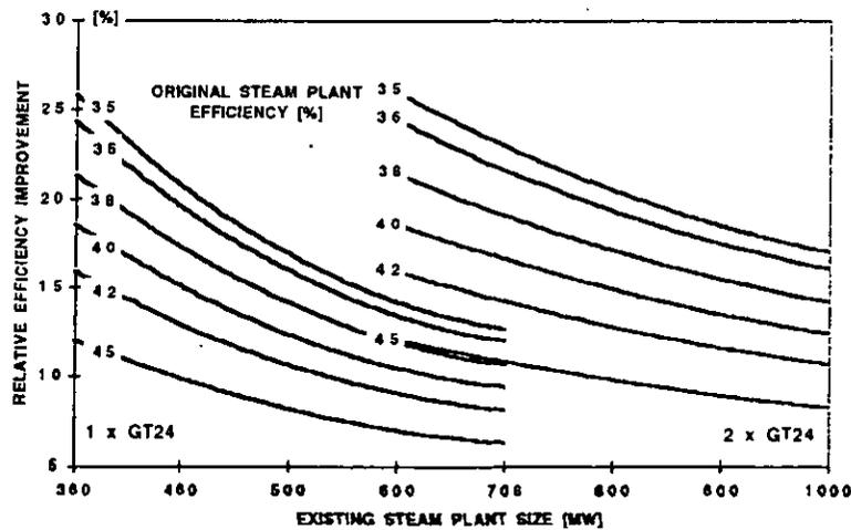
Fig. 6 - Conversion of existing CSPPs / 60 Hz with one or two GT24 : efficiency improvement versus steam plant output and current efficiency .
