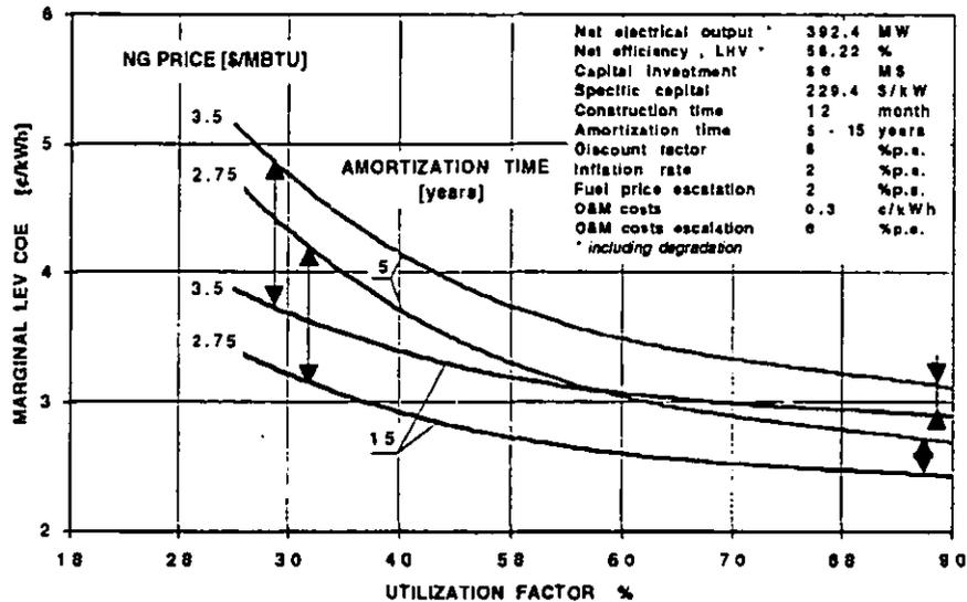
Fig. 13 - The Natural Gas Marginal LEV COE vs. utilization factor for different amortization periods (5 and 15 years).
