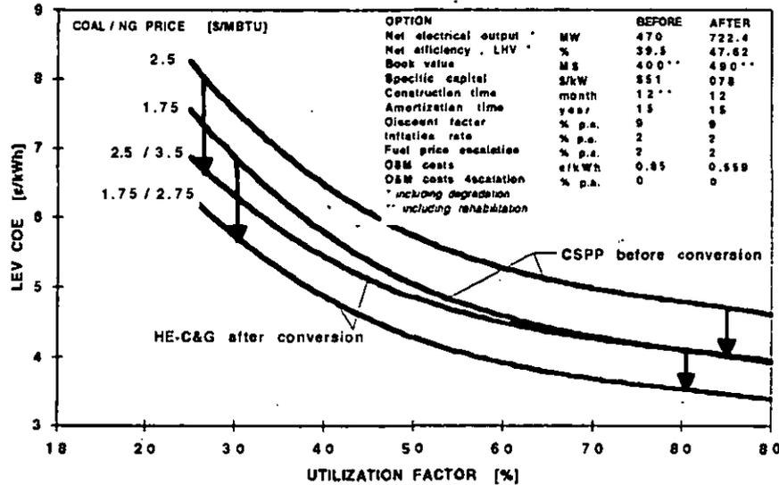
Fig. 12 - Levelized generating costs (LEV COE) before and after conversion into HE-C&G versus utilization factor .
