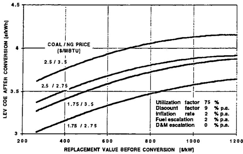
Fig. 9 - Levelized generating costs after conversion into HE-C&G with 1xGT26 of a 500 MW CSPP with different Replacement values .
