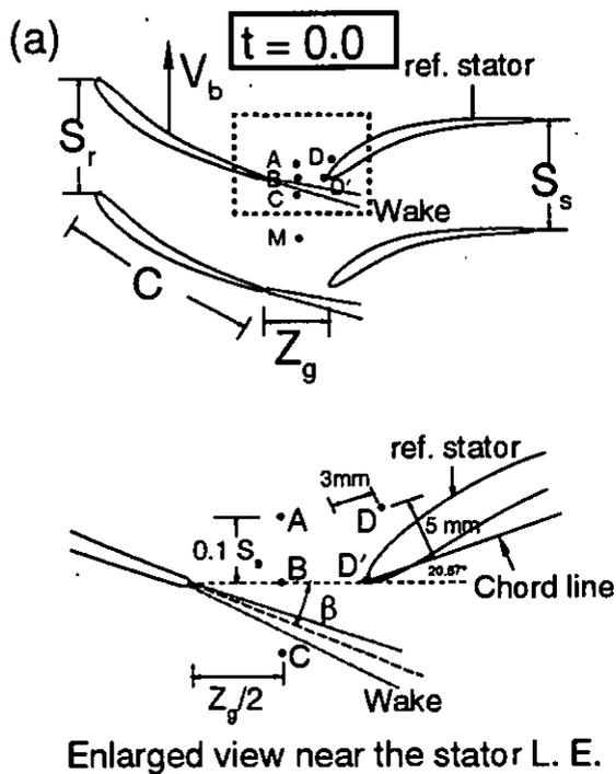
Fig. 8 A sketch of the relative position between the rotor and the stator. Figure 8a shows the time when the rotor trailing edge is axially upstream of the stator leading edge, at time  $t = 0.0$ . Also shown are hot-wire locations for gust measurement, with the view enlarged for clarity. Figure 8b shows the time when the rotor wake arrives at the stator leading edge.
