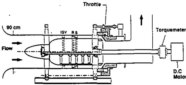
Fig. 1 The experimental compressor in IGV/rotor/stator configuration.
