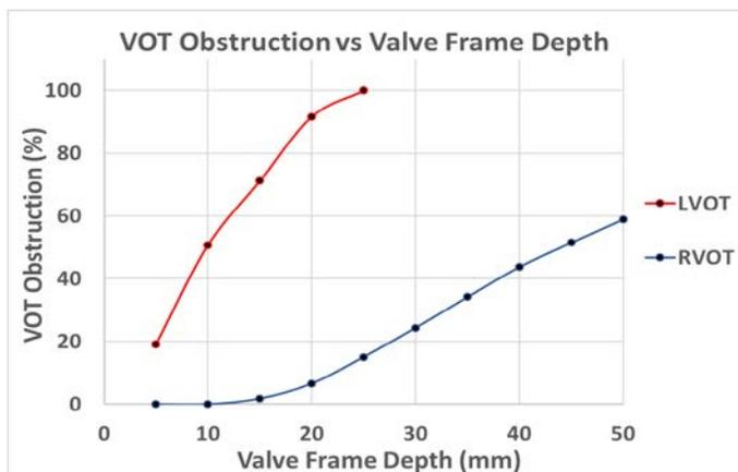
Figure 4: LVOT (red) and RVOT (blue) obstruction plots for increasing valve frame depths.
