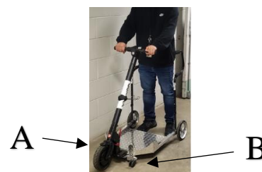
FIGURE 2. MANUAL MODE (A) FRONT WHEEL RAISED (B) CASTERS ON GROUND
