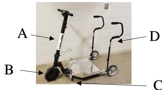
FIGURE 1. RIDING MODE. (A) STEM WITH BATTERY (B) DRIVE WHEEL (C) CASTER/ANTI-TIP WHEEL (D) HANDLES FOR MANUAL MODE
