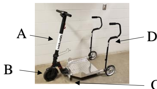
FIGURE 1. RIDING MODE. (A) STEM WITH BATTERY (B) DRIVE WHEEL (C) CASTER/ANTI-TIP WHEEL (D) HANDLES FOR MANUAL MODE
