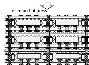
**FIGURE 7:** Fabrication process flow diagram of multi-stack die WABE package
