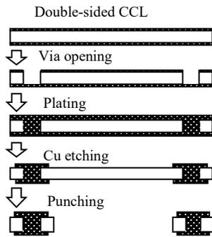
**FIGURE 5:** Fabrication process flow diagram of double-sided FPC
