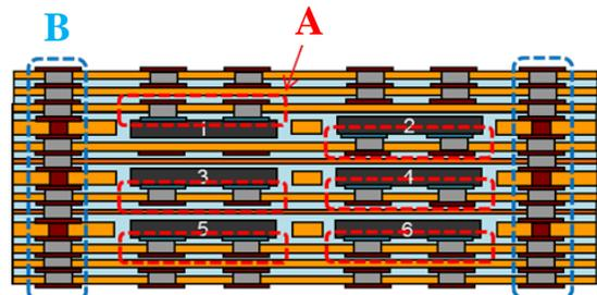
**FIGURE 9:** Electrical paths of multi-stack die WABE package
