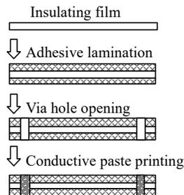
**FIGURE 6:** Fabrication process flow diagram of intermediate layer
