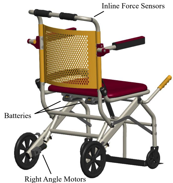
FIGURE 5: DEPICTION OF MOTOR, BATTERY, AND HANDLEBAR FORCE SENSOR PLACEMENT
