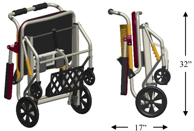
FIGURE 2: CAREGIVER-ASSIST TRANSPORT CHAIR IN FOLDED CONFIGURATION
