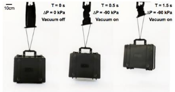
Figure 6: Lifting test (5.5 kg) of soft origami from the exerted force of pump.
