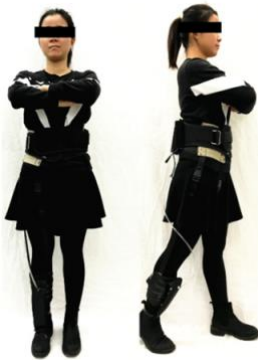
Figure 9: A subject wearing the prototype of the vacuum-driven soft wearable robot for ankle assistance.
