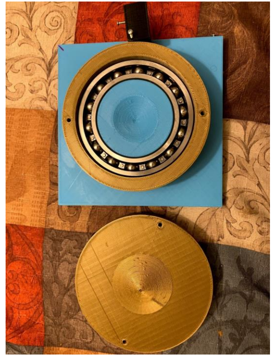
FIGURE 2: Final assembly with smartphone (a). The top plate is removable (b) and is easily replaceable for sample loading. A Nexus 5X was utilized for the smartphone that is affixed to the top plate. For a sense of scale, the base plate measures 20 cm x 20 cm and the entire device has a height of 7.5 cm not including the smartphone.
