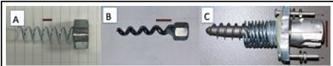
Figure 1: Examples of the three primary prototype designs. (A) Single flexible coil preliminary design (Length: 4.818 cm, Diameter: 2.54 cm, Pitch: 0.569 cm). (B) Single helix stiff coil mechanical prototype made using corkscrew (Length: 5 cm, Diameter: 1.735 cm, Pitch: 0.900 cm). (C) Hybrid two-part mechanical prototype with a custom grip that allowed for screws to attach and simultaneously engage both parts of the state, leading to combined tension throughout the device.
