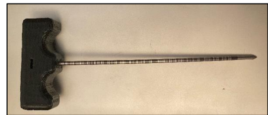
Figure 5: The modified Jamshidi instrument is shown here. The etched guide wire used with the simulator tracking system was able to be press fit into the 3D printed handle.
