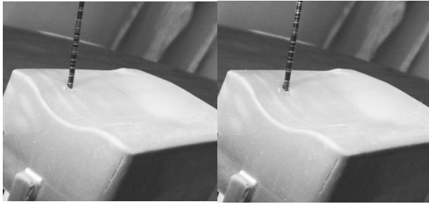
Figure 9: The left image shows the wire on the simulator before any hammering of the Jamshidi handle. The right image shows the wire after it had been hammered into the spinal body, still is sharp focus.
