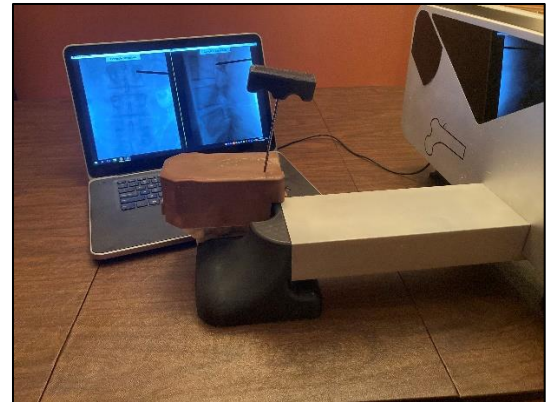
Figure 7: The new spine model is shown mounted to the simulator. The Jamshidi handle has been placed into the silicone soft tissue, and images reconstructed on the laptop accurately show the wire on the spine model surface.
