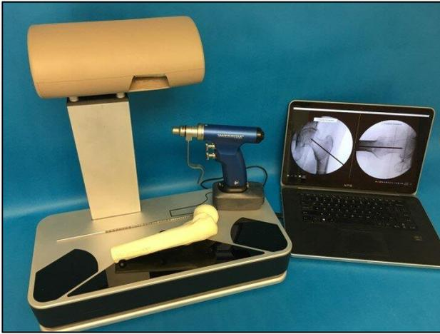
**Figure 1:** The current wire navigation simulator platform for hip wire placement. A laser etched K-wire is tracked as it is advanced into a surrogate femur bone, with an associated laptop presenting virtual fluoroscopic images for navigation.
