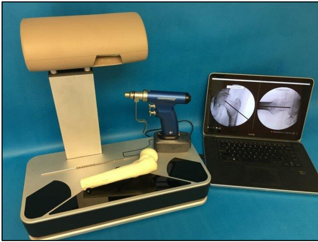
Figure 1: The current wire navigation simulator platform for hip wire placement. A laser etched K-wire is tracked as it is advanced into a surrogate femur bone, with an associated laptop presenting virtual fluoroscopic images for navigation.
