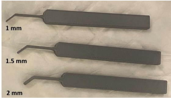
FIGURE 3: MEASURING TOOLS. THE TOOLS WITH A SPECIFIC THICKNESS AT THEIR TIP HAVE BEEN 3D PRINTED TO DETERMINE THE AVAILABLE SPACE BETWEEN THE ARTICULATING SURFACE OF METACARPAL AND PROXIMAL PHALANX OF THE THUMB.
