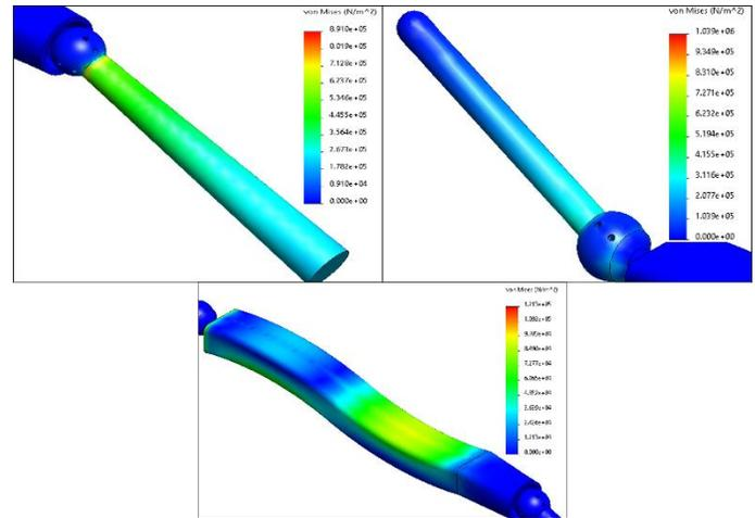
**FIGURE 5:** Stress analysis results of intrauterine arm, body, and handle (from top to bottom), showing where the most amount of deformation can occur at each tested part.
