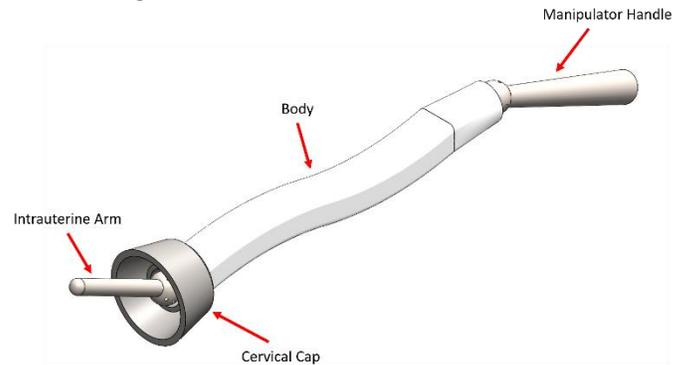
**FIGURE 3:** CAD model of the proposed uterus manipulator design.
