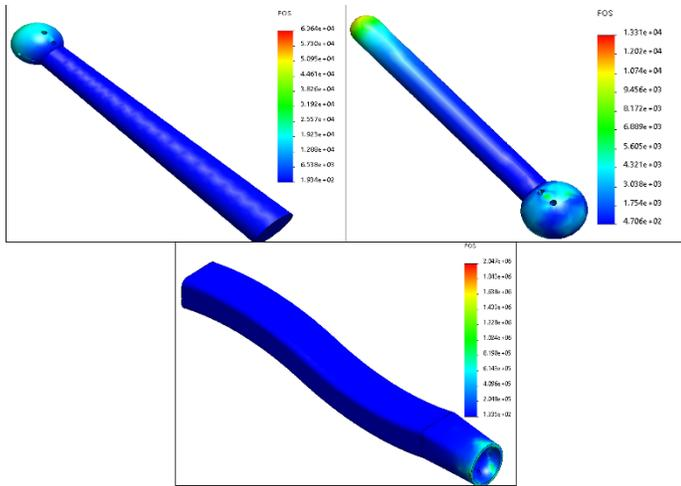
**FIGURE 6:** Factor of Safety analysis results of intrauterine arm, body, and handle (from top to bottom), showing where the most amount of deformation can occur at each tested part.
