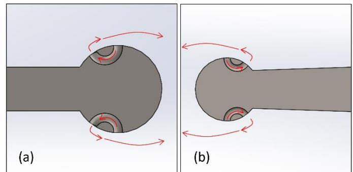
**FIGURE 4:** Cross-sectional view of the ball joint hole curvature in the intrauterine arm (a), and handle (b).
