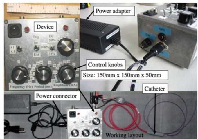
FIGURE 1: BENCHTOP EUCD AND WORKING LAYOUT
