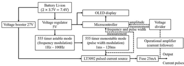
**FIGURE 2: MECHATRONIC EUCD SCHEMATIC AND SIGNAL FLOW DIAGRAM**
