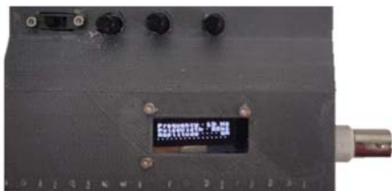
FIGURE 4: MECHATRONIC EUCD PROTOTYPE WITH AND OLED PLACED IN A 3D PRINTED ENCLOSURE
