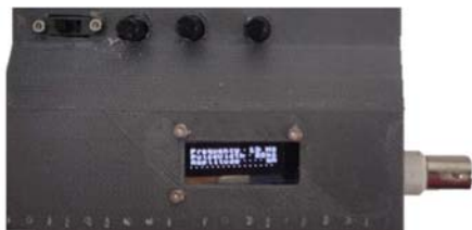
FIGURE 4: MECHATRONIC EUCD PROTOTYPE WITH OLED PLACED IN A 3D PRINTED ENCLOSURE
