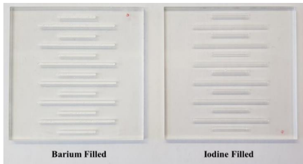
FIGURE 1: Radiopaque scale design with filled with two separate agents.
